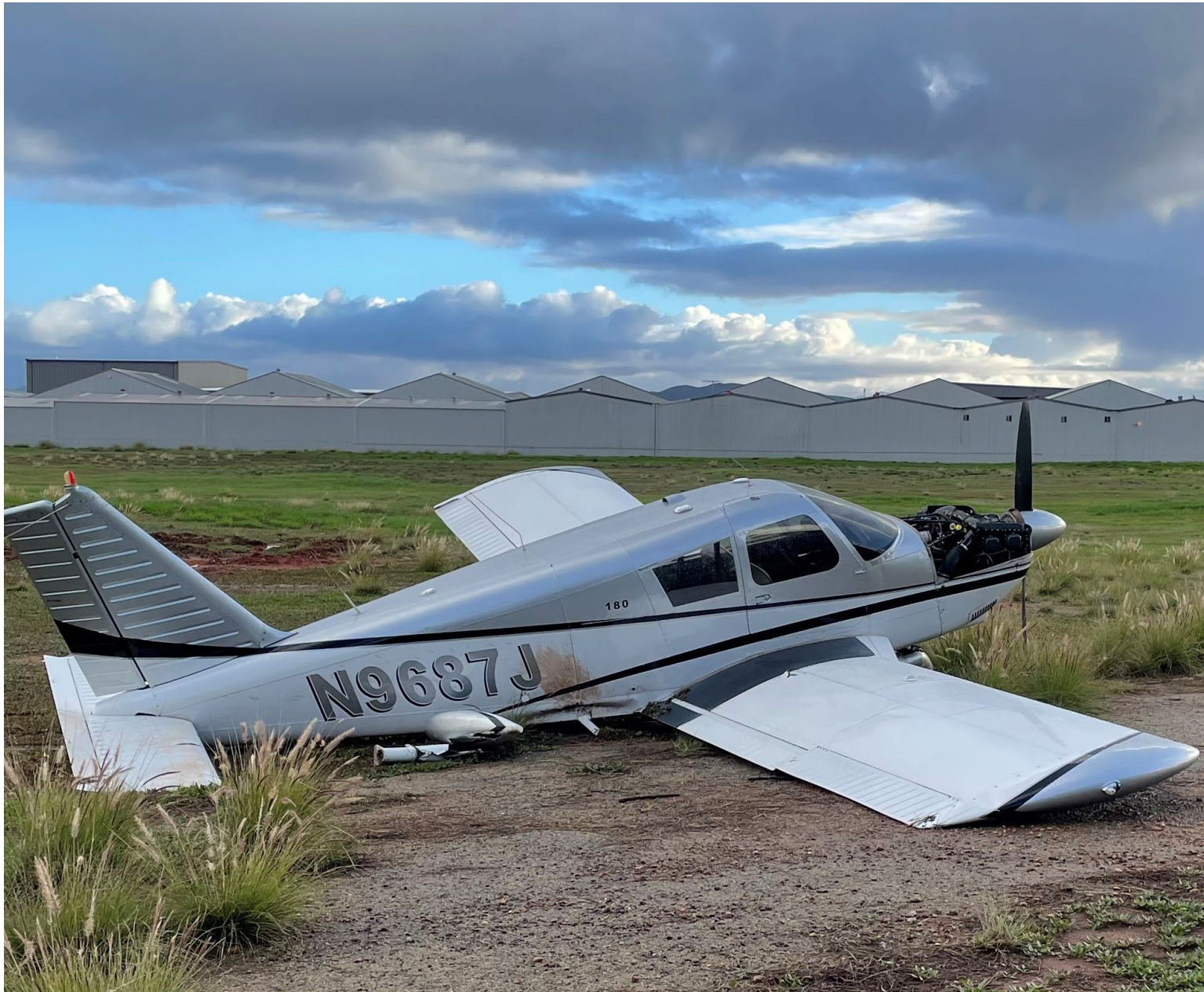
Photo 1 – View of substantial damage to fuselage (photo courtesy of pilot)
