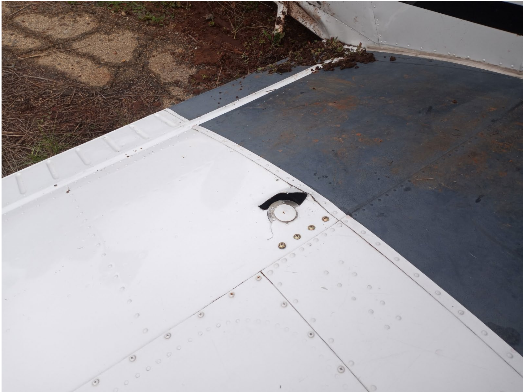
Photo 2 – View of substantial damage to right wing (photo courtesy of pilot)
