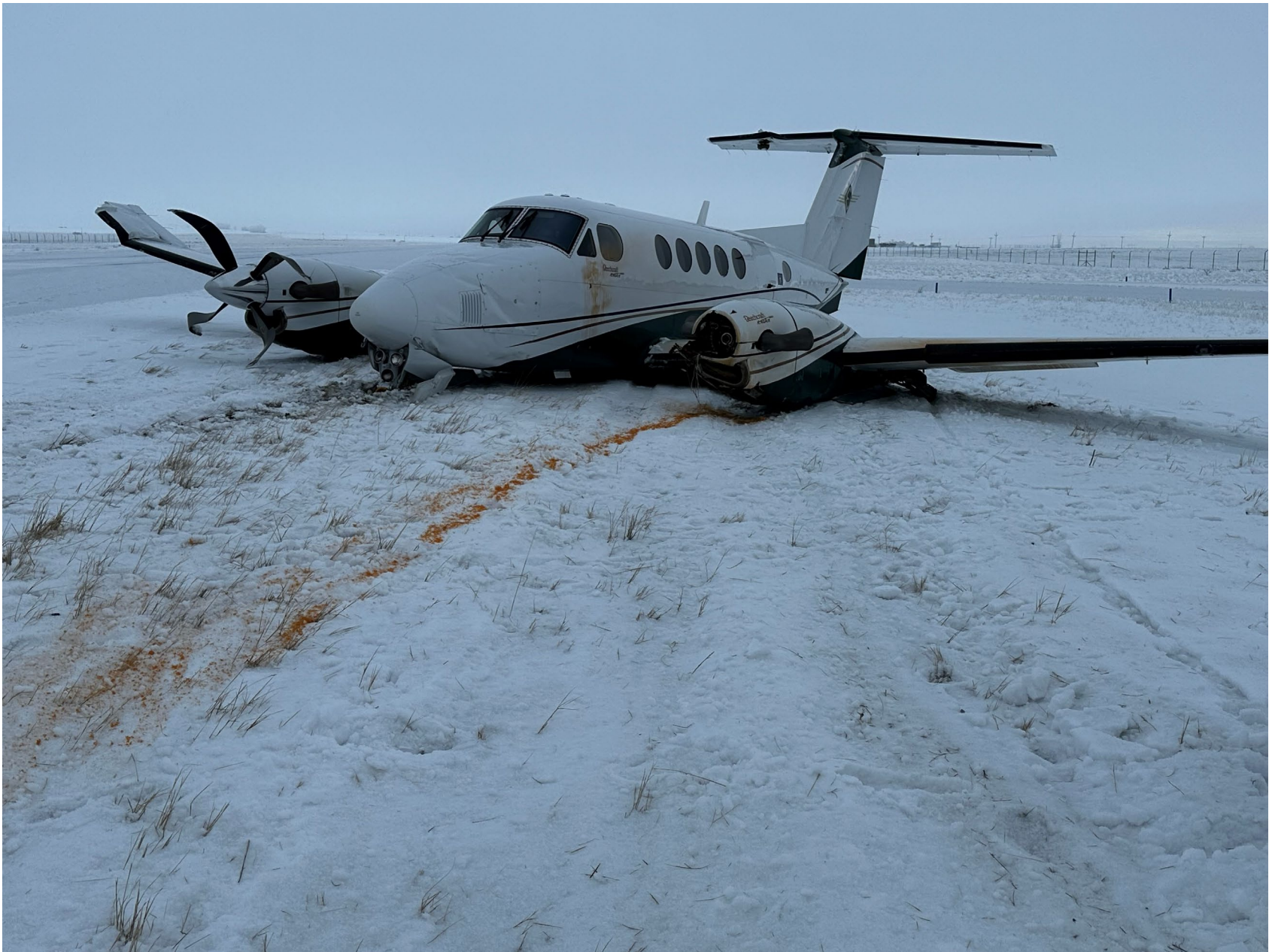
Photo 1 – Forward view of airplane damage. (Photo courtesy of airport manager)
