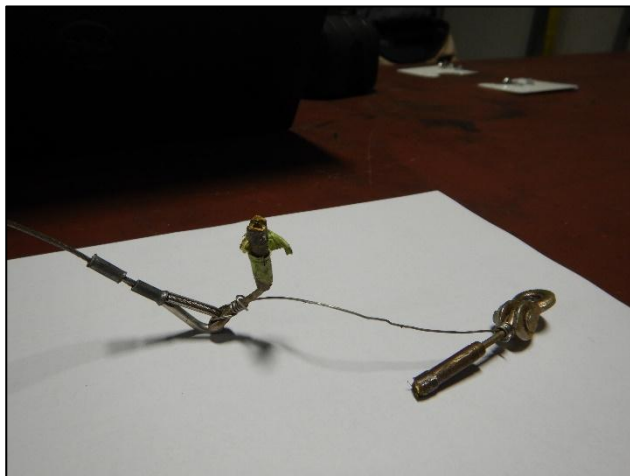
Figure 15-Left aileron cable at the forward stick position.
