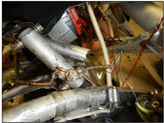
Figure 14-Forward control stick and aileron cable attachments.
