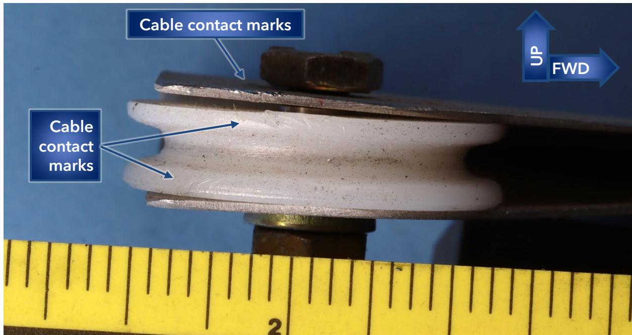
Figure 3. Cable contact marks on the sides of the pulley groove and on the inboard edge of the upper bracket.
