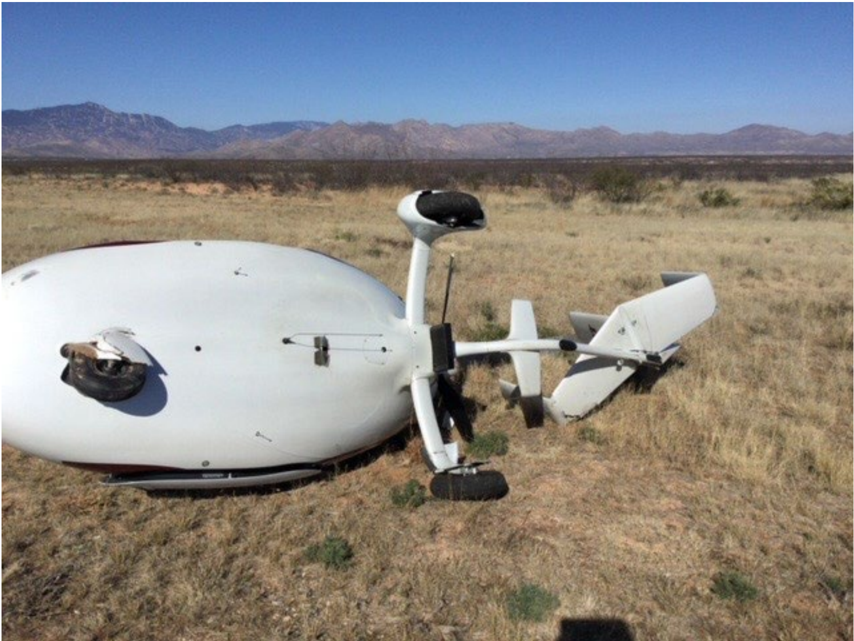
Photo 1 – View of Fuselage, Tail Boom and Horizontal Stabilizer Damage (Courtesy of Pilot)
