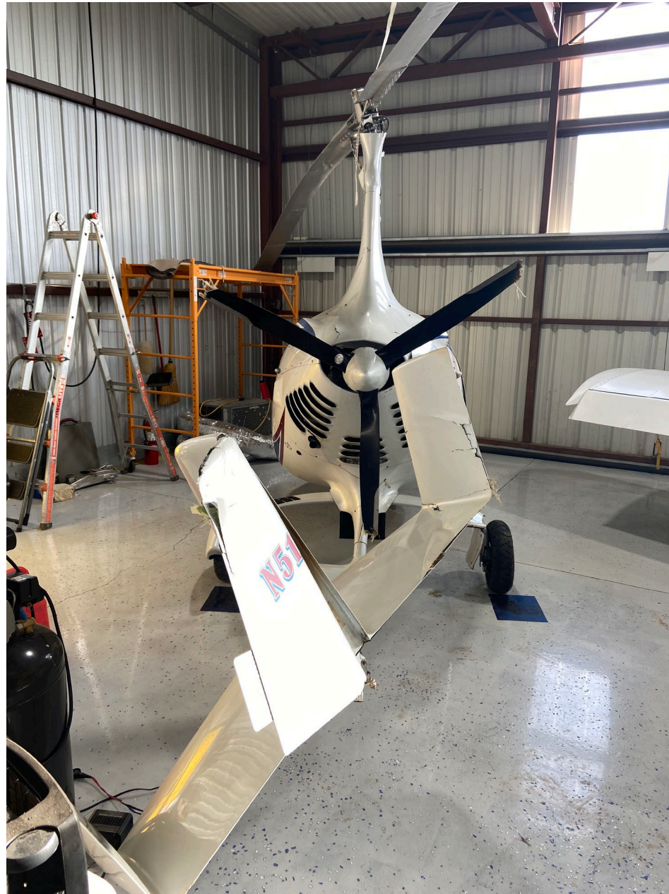
Photo 2 – View of Horizontal Stabilizer and Rudder Damage (Courtesy of FAA)
