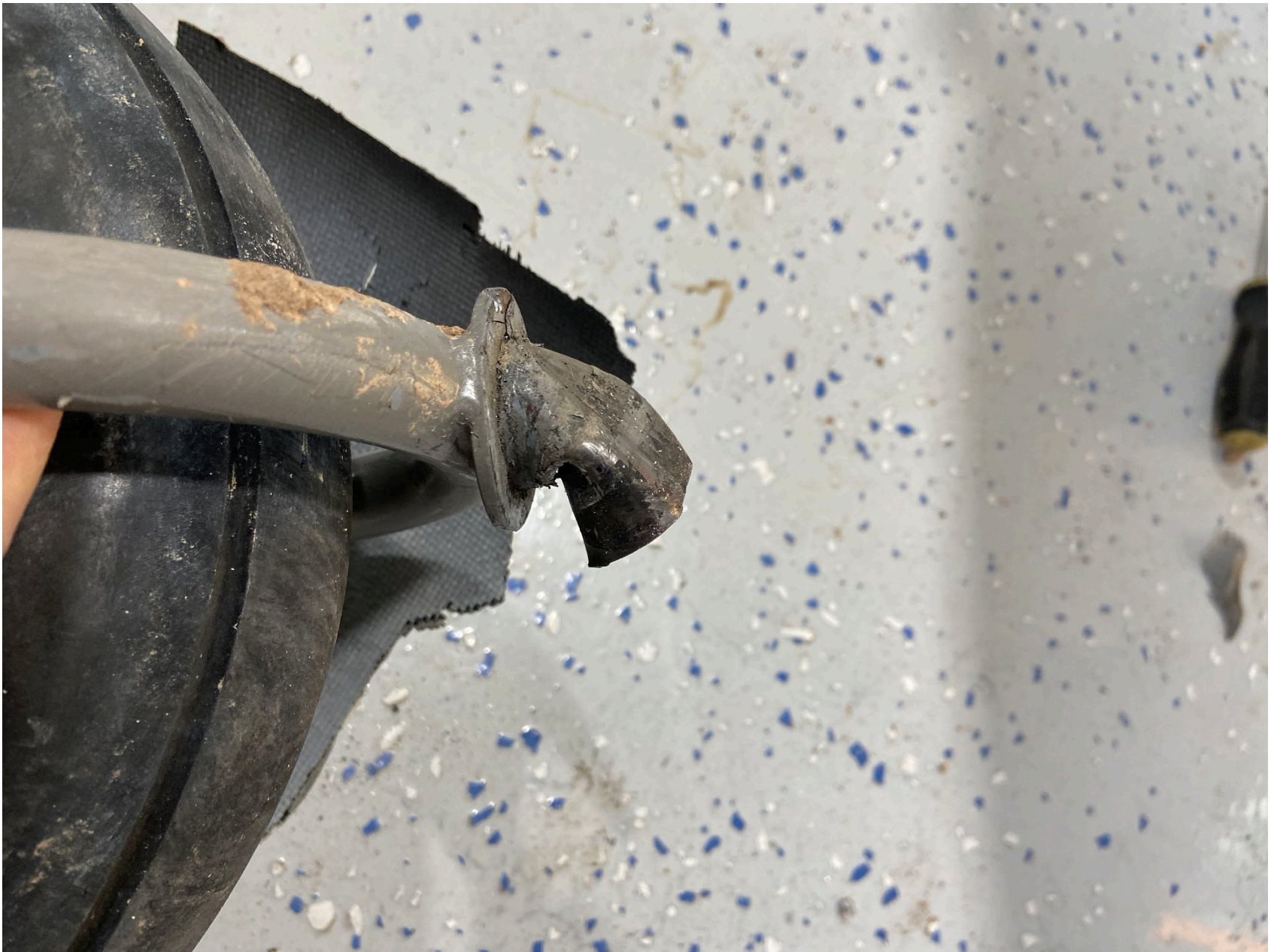
Photo 3 – View of Nose Strut Damage (Courtesy of FAA)
