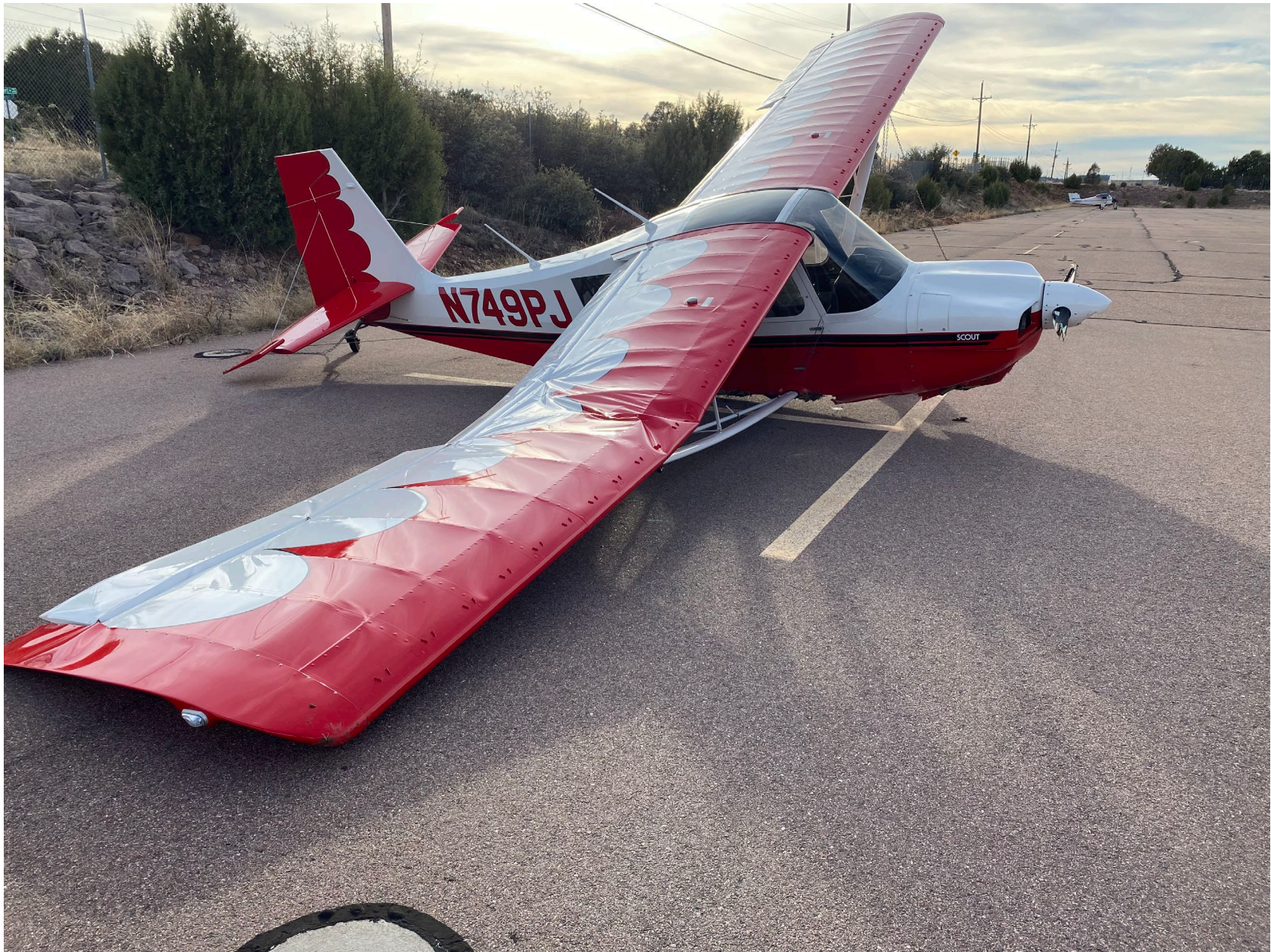
Photo 1 – View of right wing damage (photo courtesy of the pilot)
