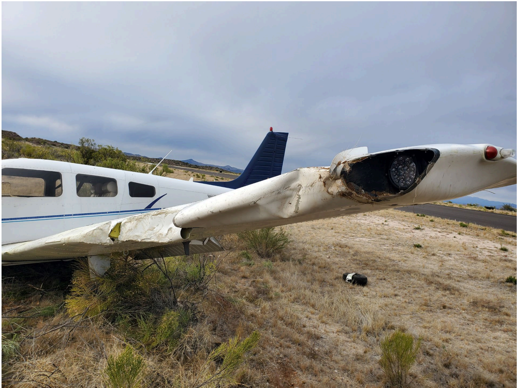
Photo 1 – View of substantial damage to left wing (photo courtesy of FAA)
