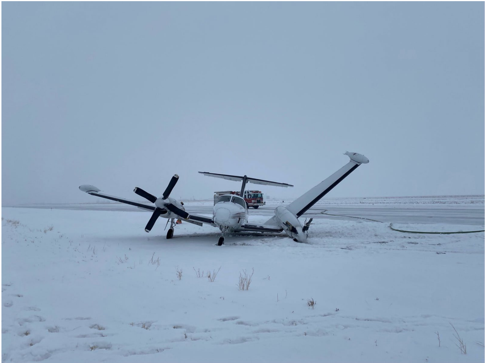
Photo 1 – View of Damage to Left Wing (Courtesy of Airport Crash Fire Rescue)
