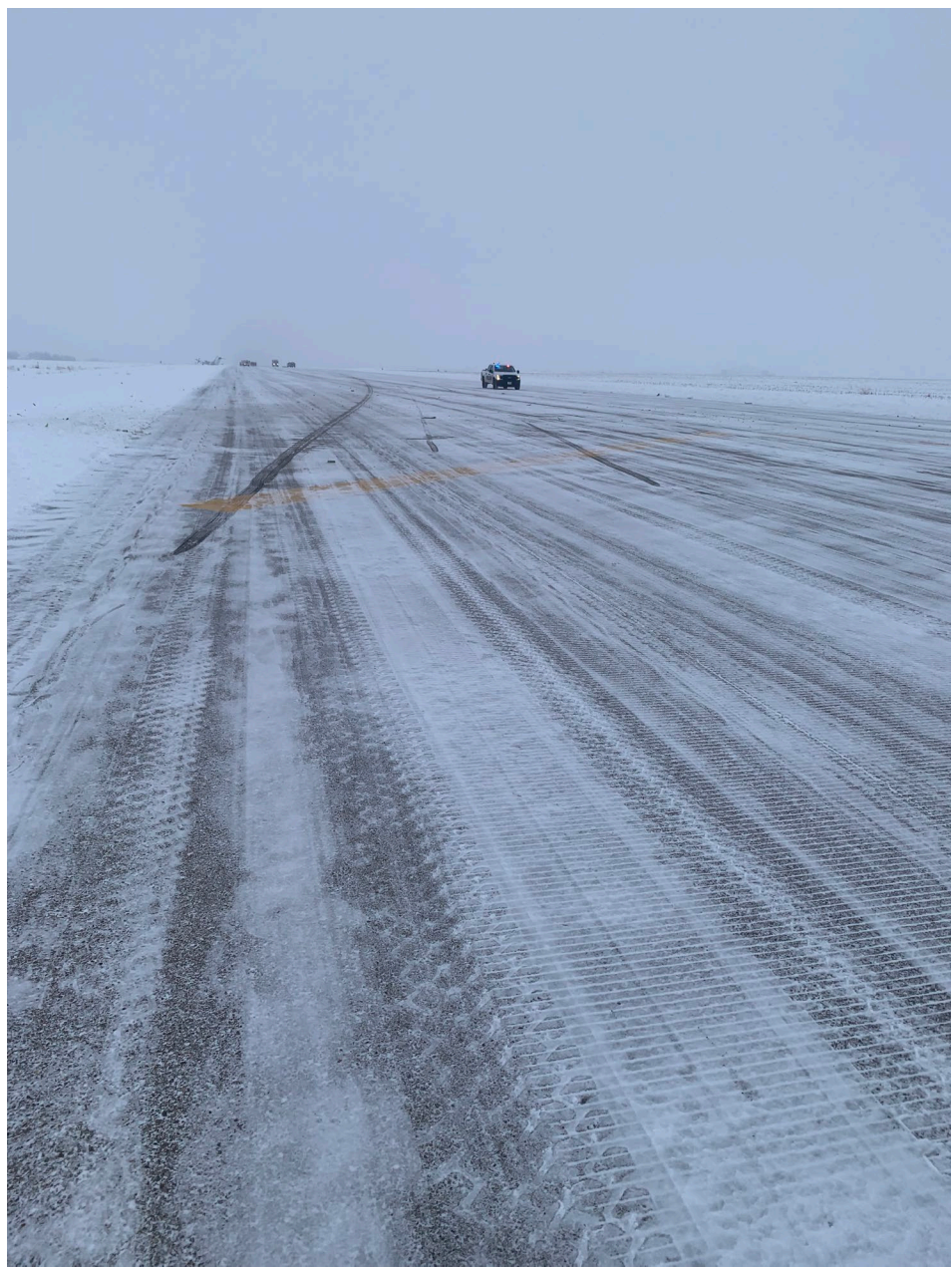
Photo 2 – View of Landing on Unusable Runway and Propellor Strikes (Courtesy of Airport Manager)
