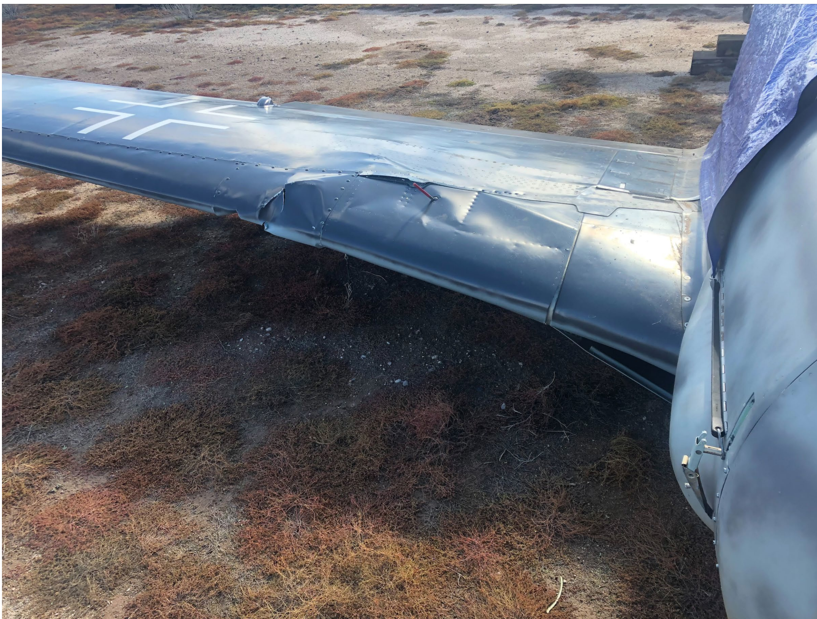
Photo 1 – View of substantial damage to right wing (photo courtesy of pilot)
