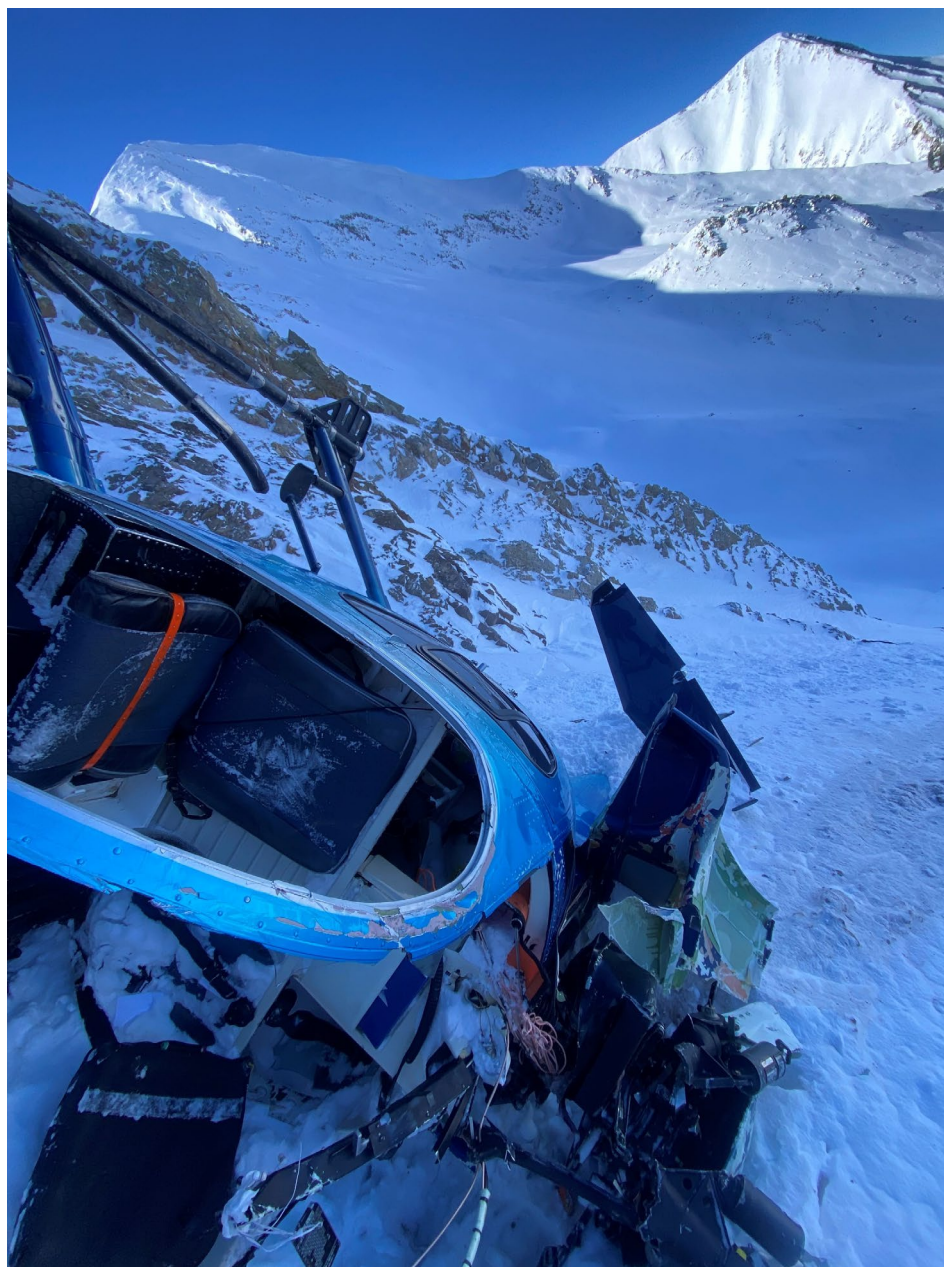
Photo 1 –N458HW front view, showing the damage to the fuselage, tail cone, and main rotor head. Photo courtesy of the operator.
