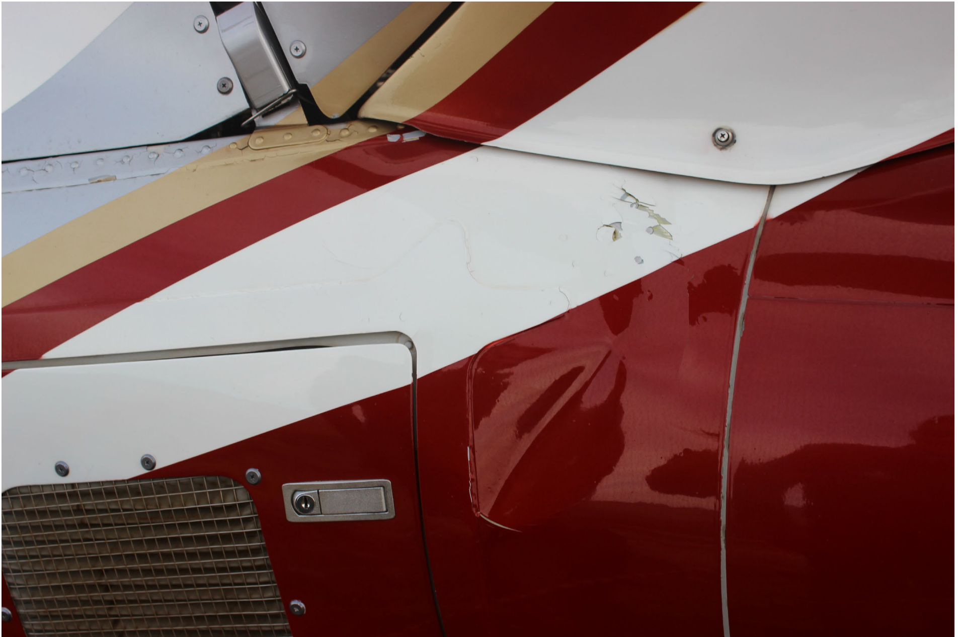
Photo 1 – Damage of apt Fuselage (photo courtesy of company)
