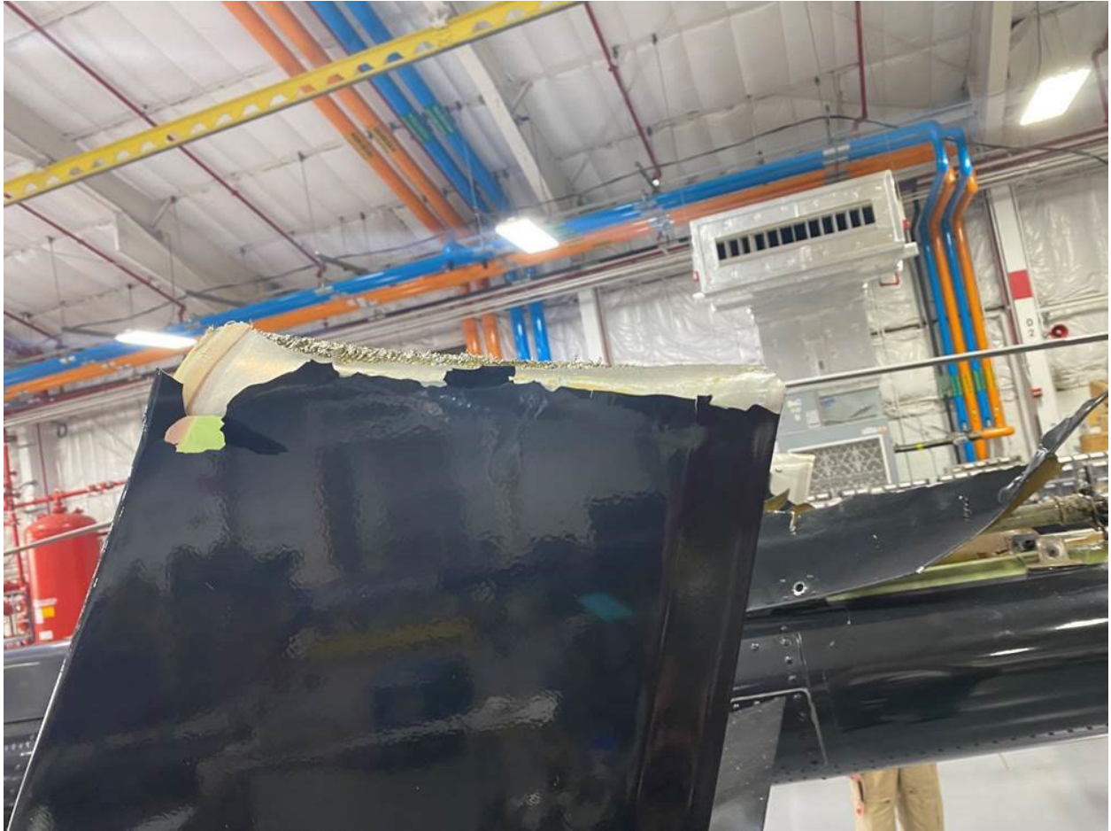
FIGURE 2 - VERTICAL FIN DAMAGE
