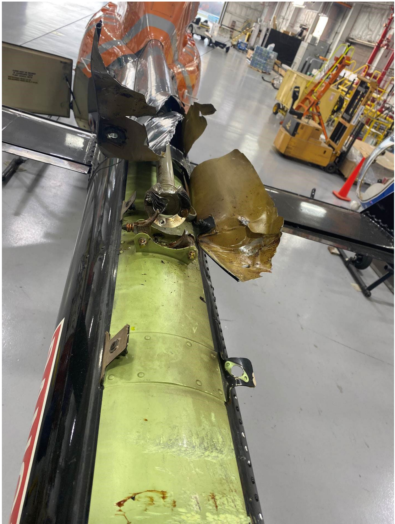
FIGURE 1 - TAIL ROTOR DRIVE SHAFT DAMAGE
