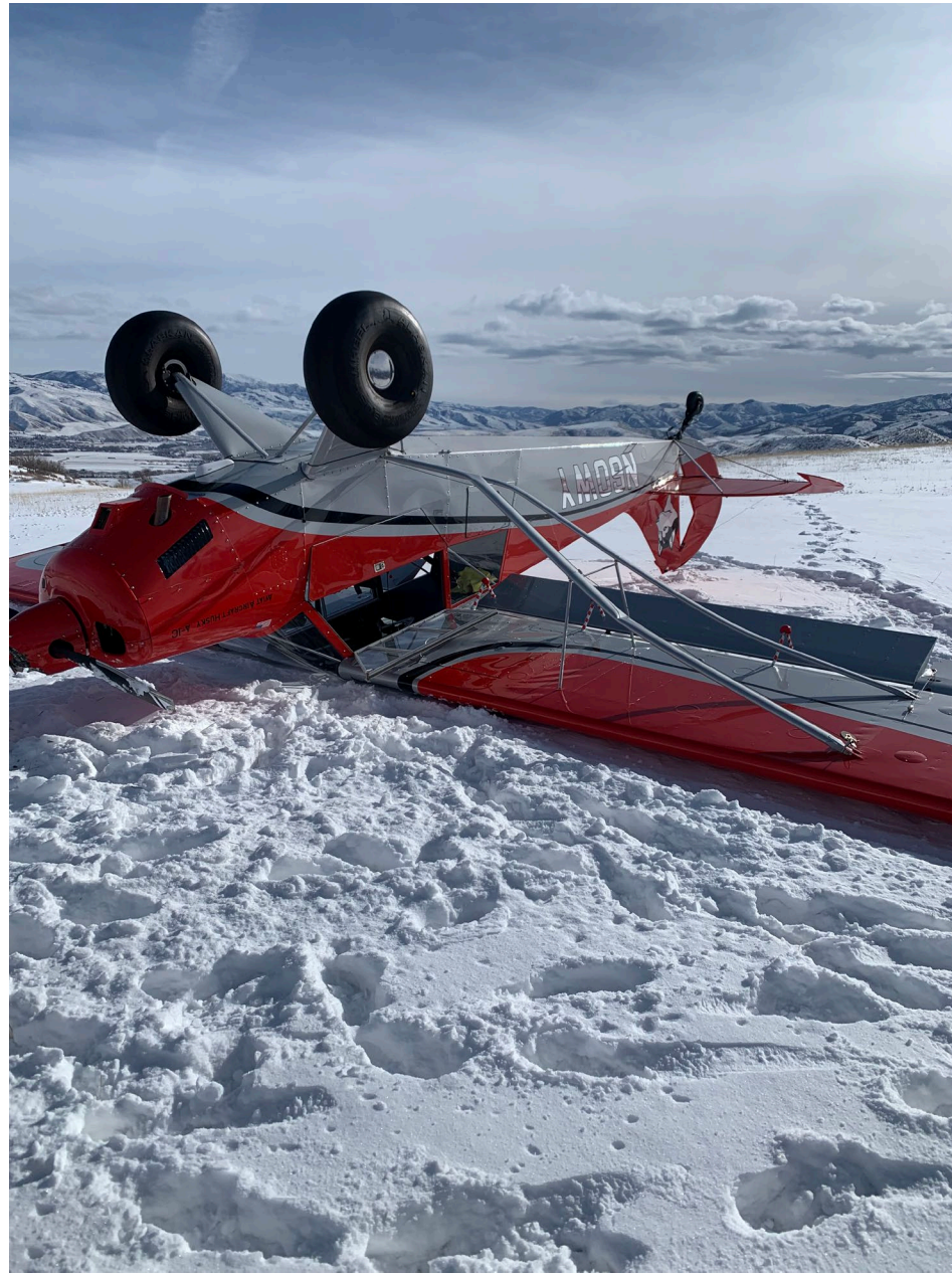
Photo 1 – View of Left Wing, Vertical Fin, and Rudder Damage (Courtesy of Pilot)
