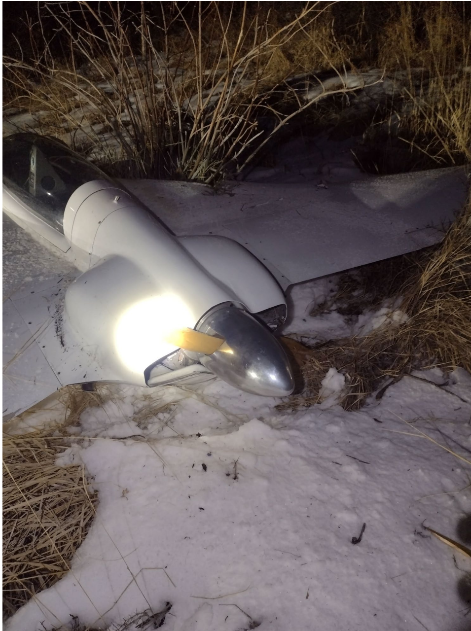
Photo 2 – view of right wing leading edge damage (photo courtesy of pilot)
