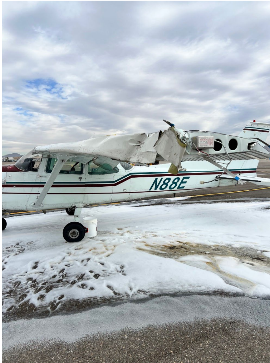
Photograph 4 - View of damage to left wing leading edge and rib (Courtesy of FAA)
