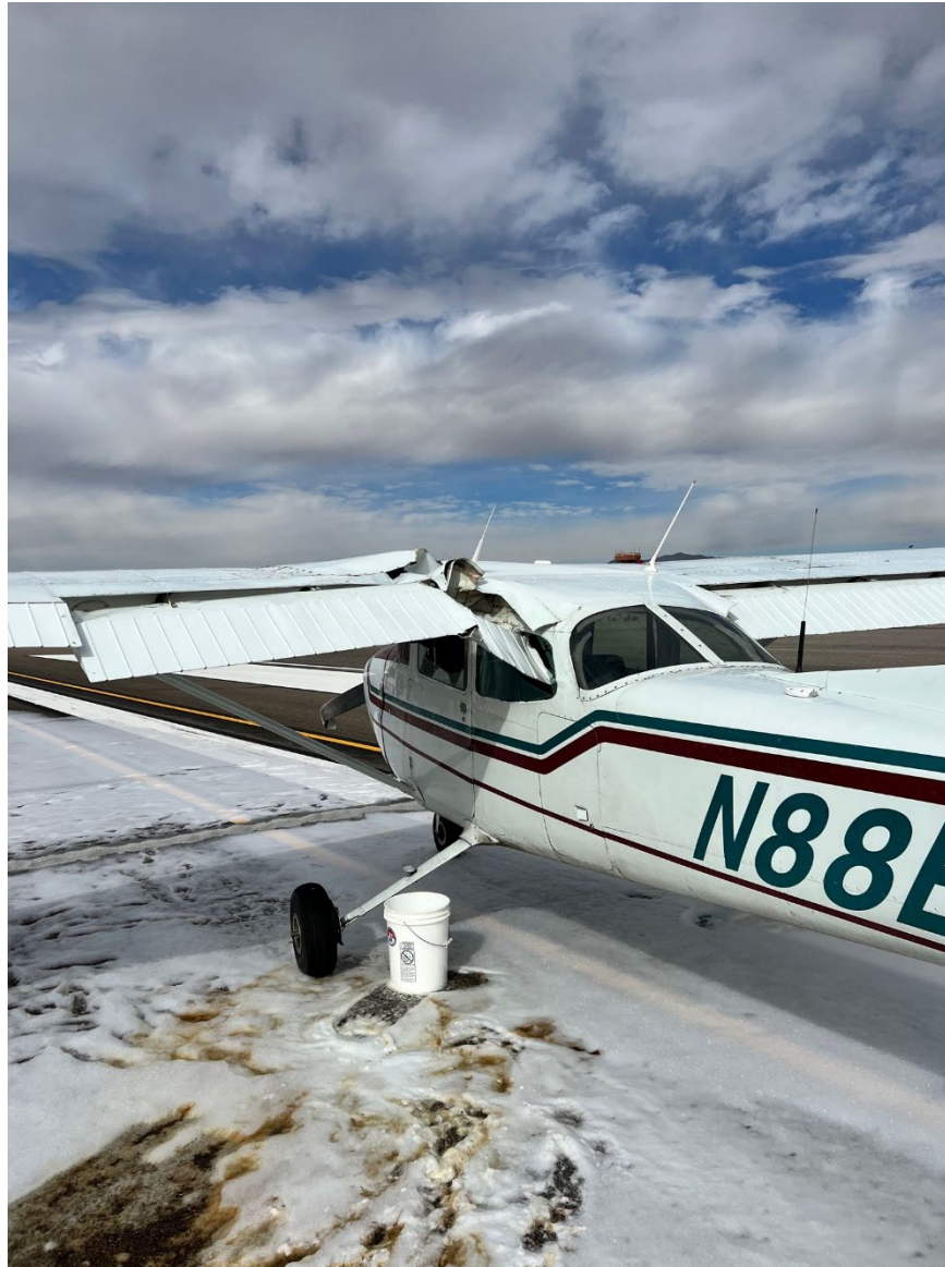
Photograph 3 - View of damage to left wing root (Courtesy of FAA)
