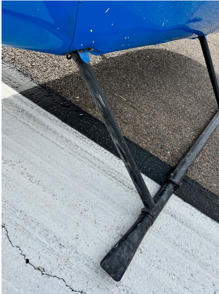
Photograph 1 - View of the initial point of impact being the aft right skid (Courtesy of FAA)
