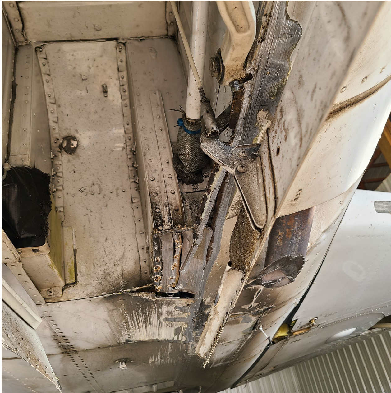
Photo 2 – View of substantial damage to belly (photo courtesy of pilot)
