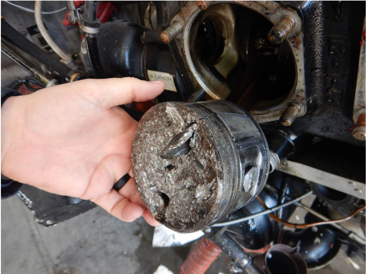
Figure 4 - No. 1 Piston with embedded Exhaust Valve and Crack
