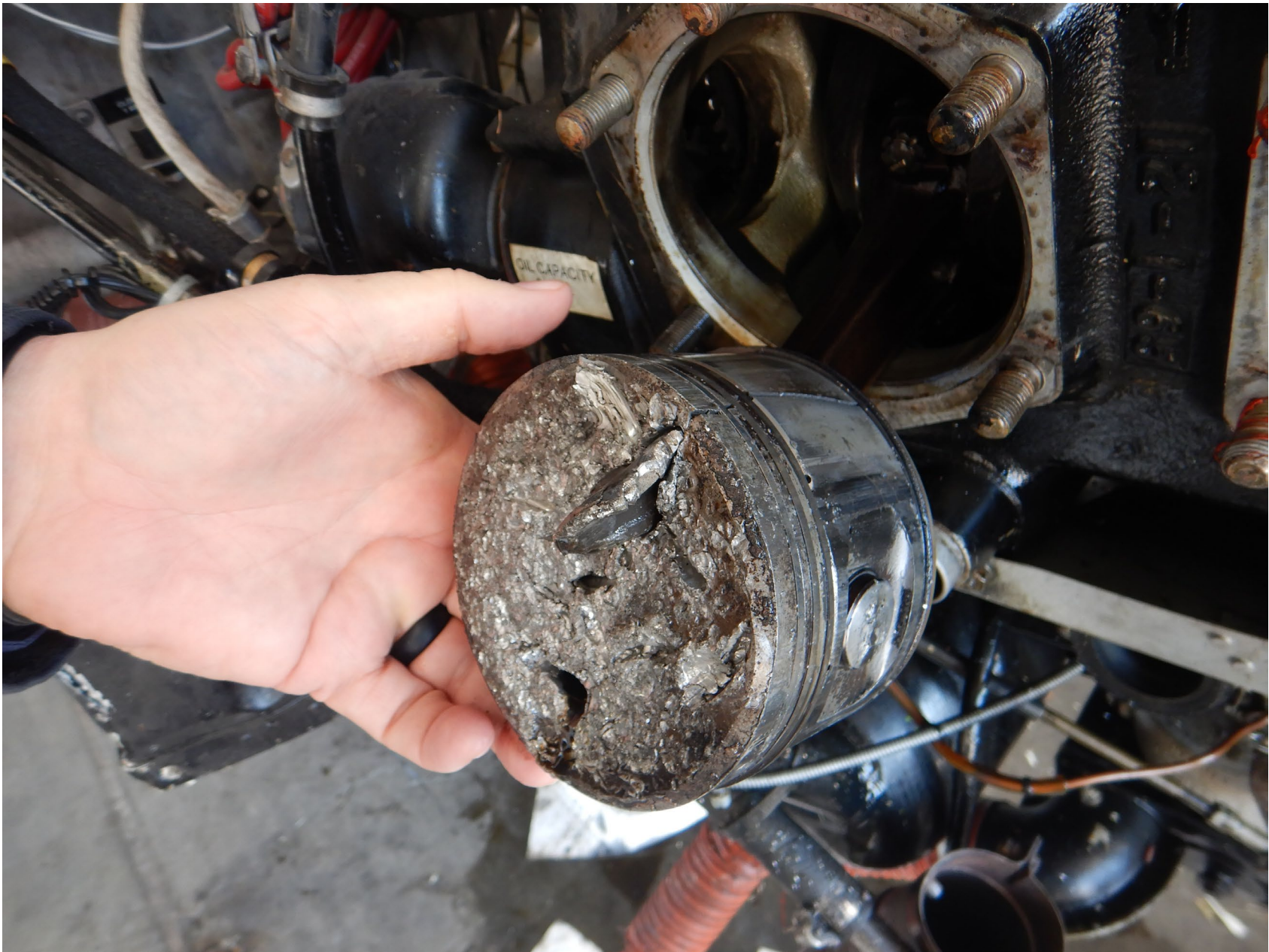
Photo 5 - No. 1 Piston with embedded Exhaust Valve and Crack
