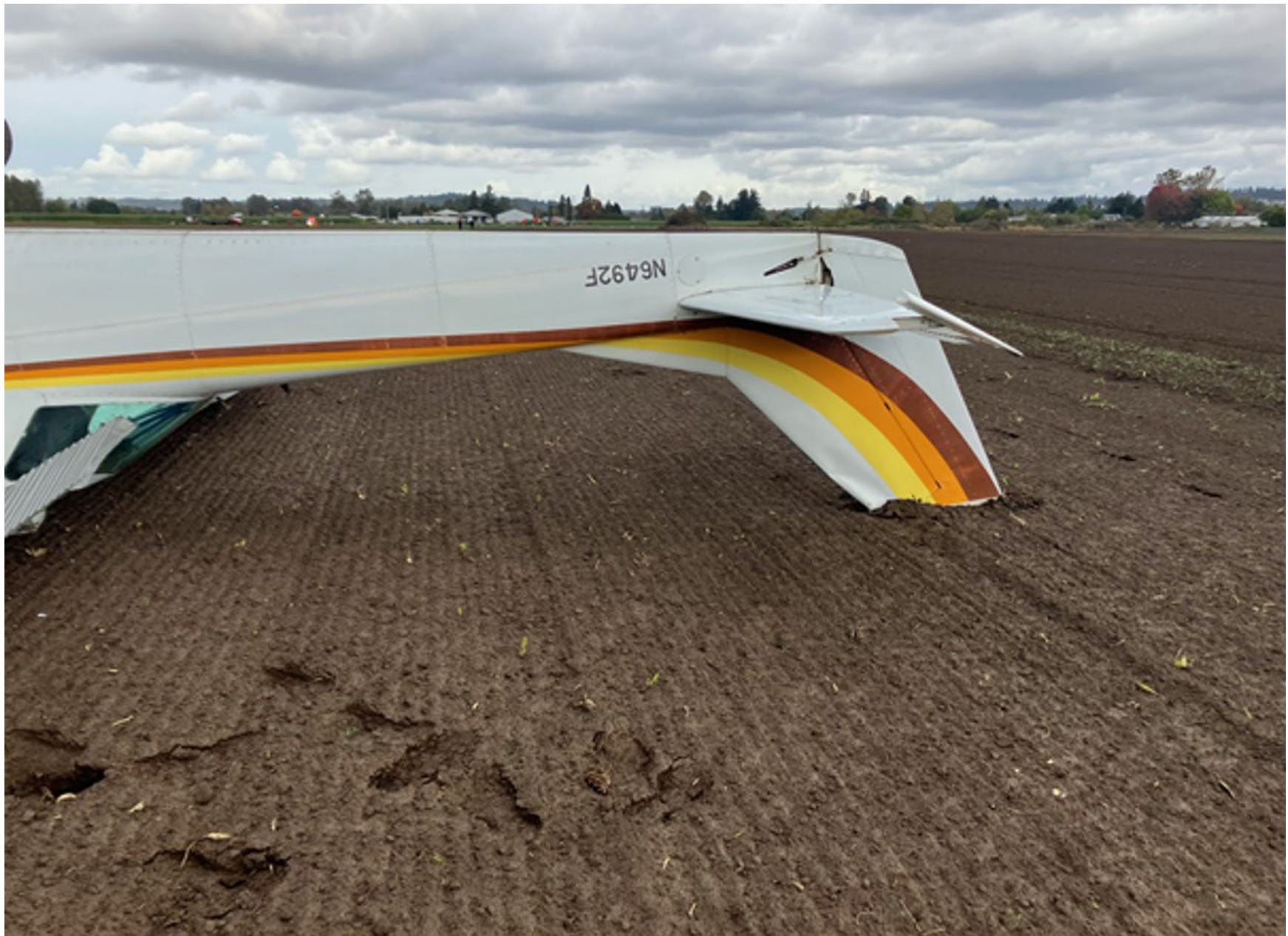
Photo 1 – photo of substantial damage to vertical stabilizer (photo courtesy of pilot)
