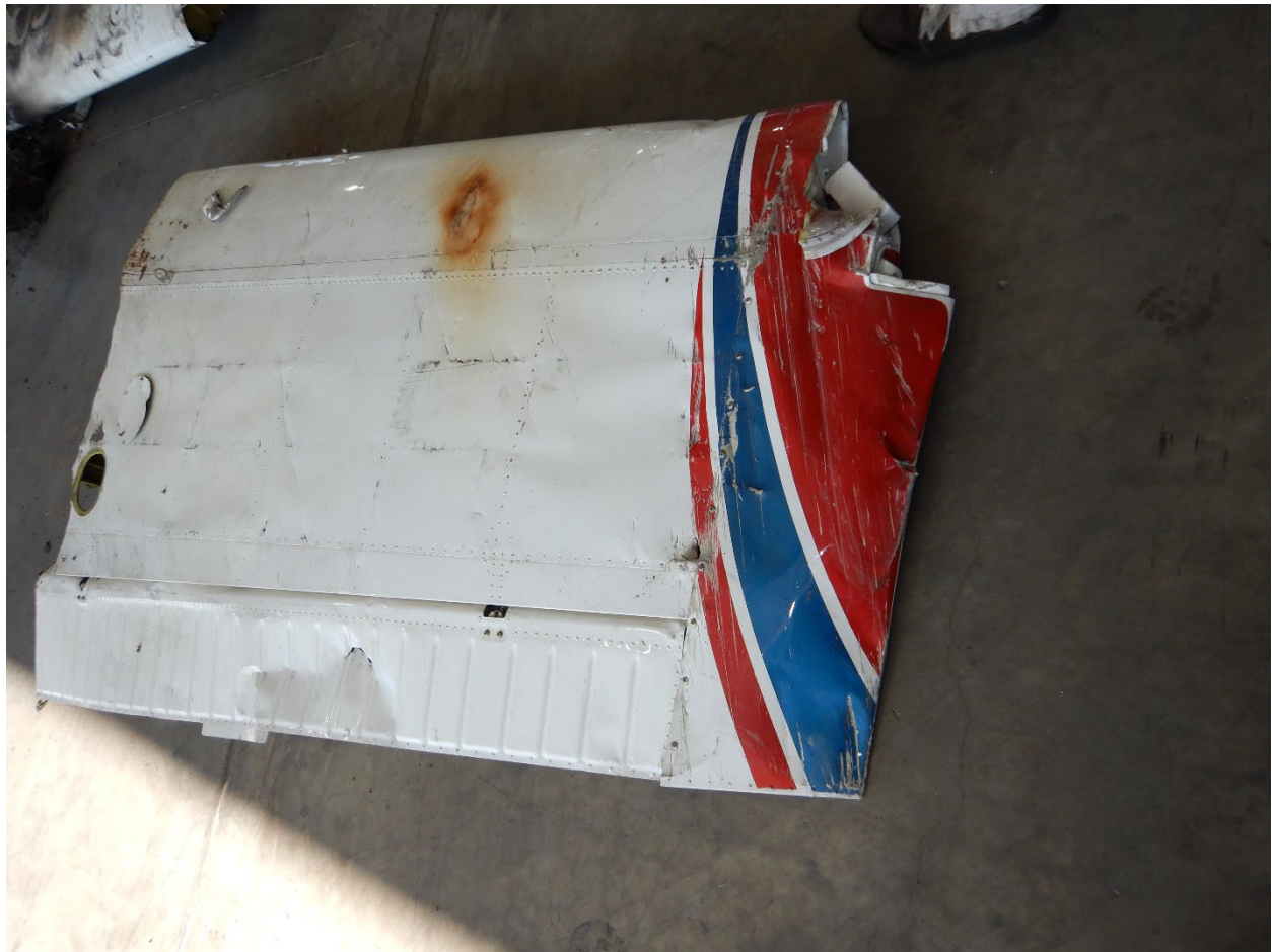
Photograph 3: Underside of left-wing tip that scraped asphalt
