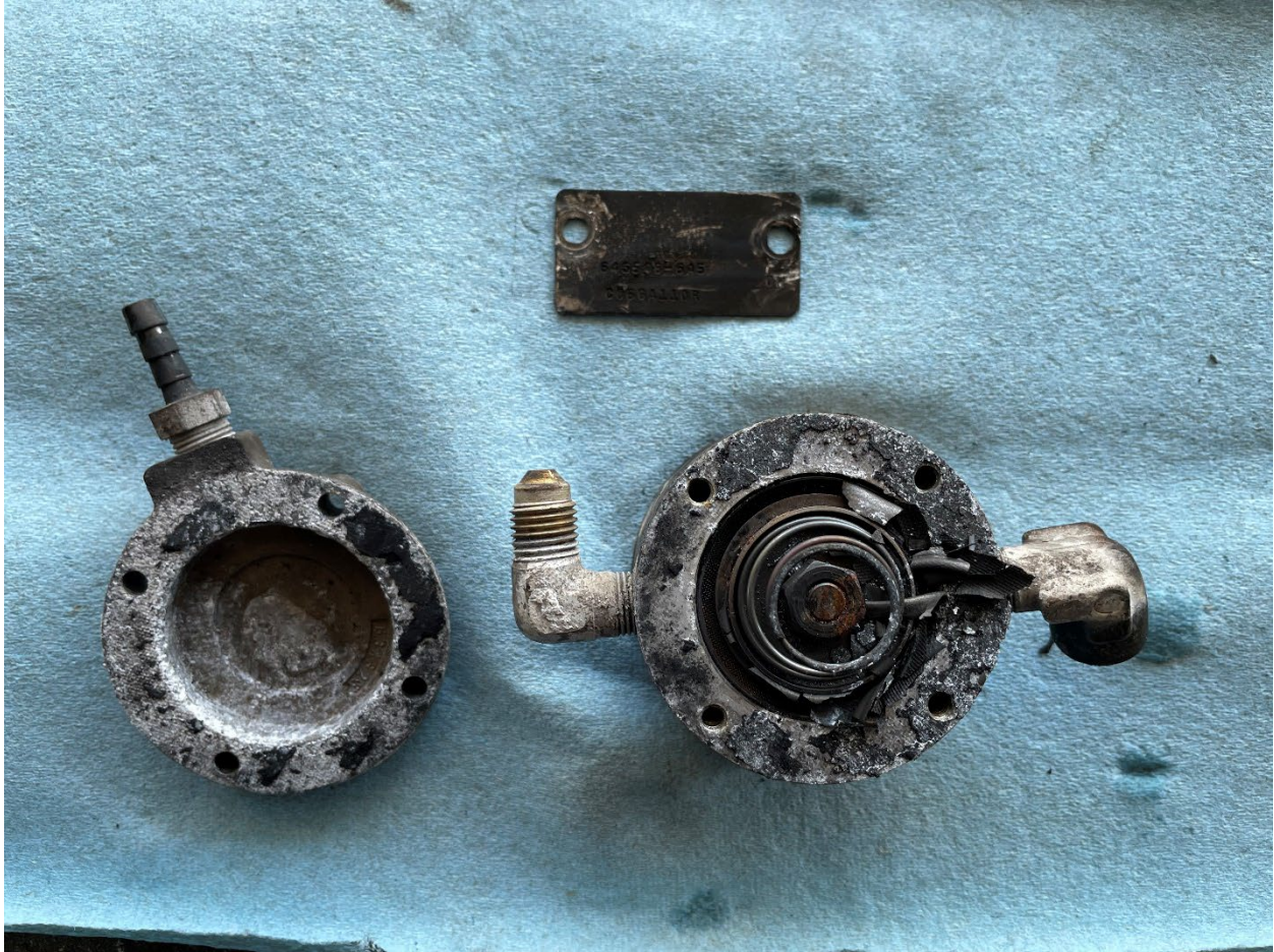
Figure 4. Close-up view of thermal damaged fuel flow divider
