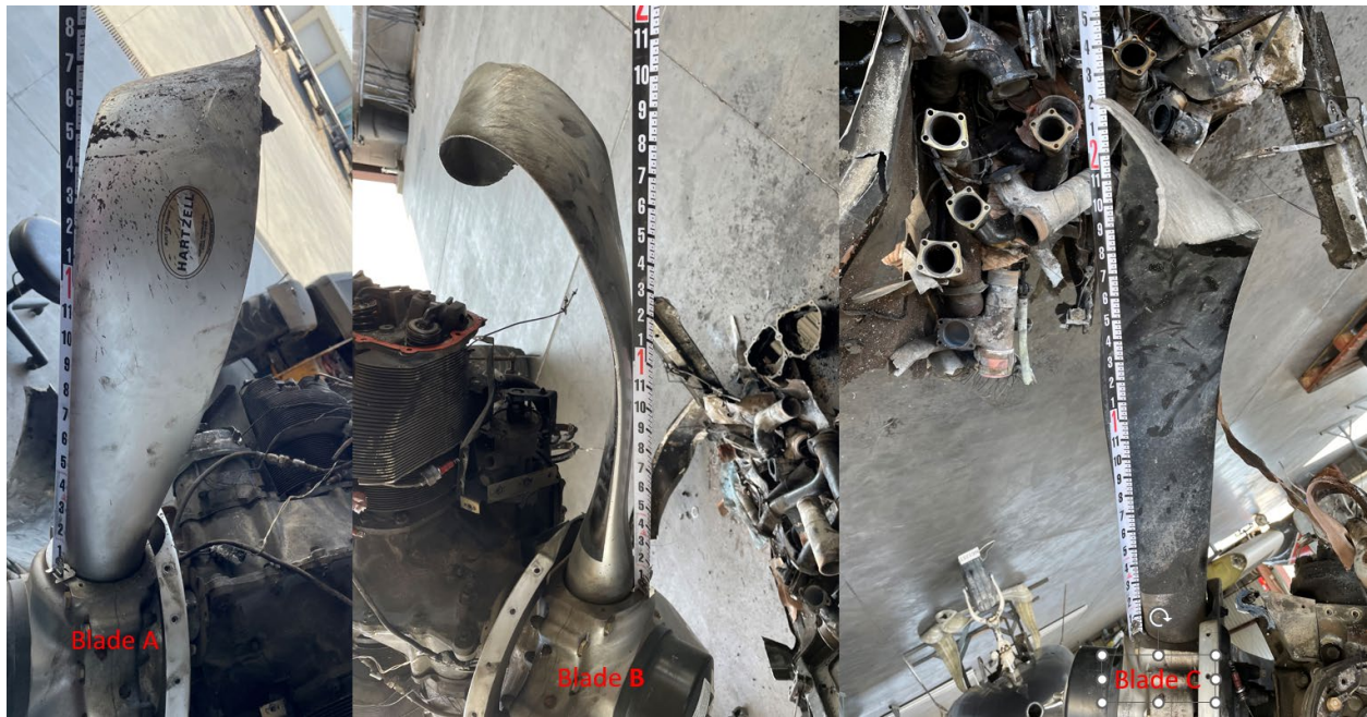
Figure 5. View of damaged propeller blades
