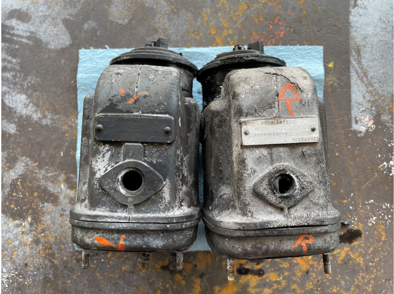
Figure 3. View of thermal damaged left and right magnetos
