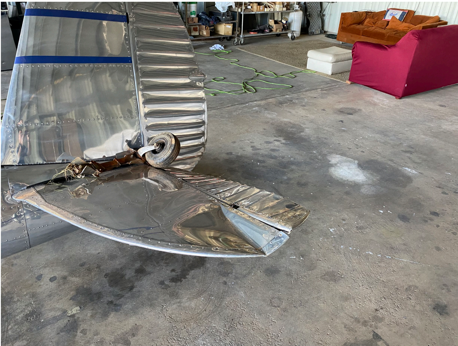
Photo 4 – Left horizontal stabilizer and elevator (courtesy of FAA)
