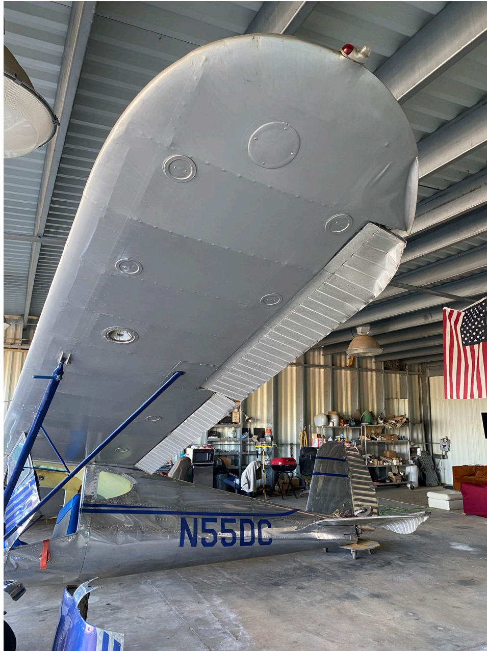
Photo 3 – Left aileron (courtesy of FAA)
