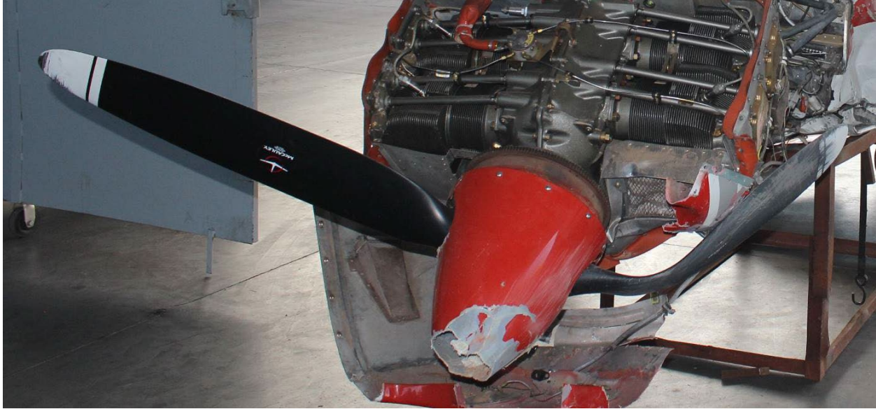
Figure 4. View of damaged propeller (photo courtesy of engine manufacturer)
