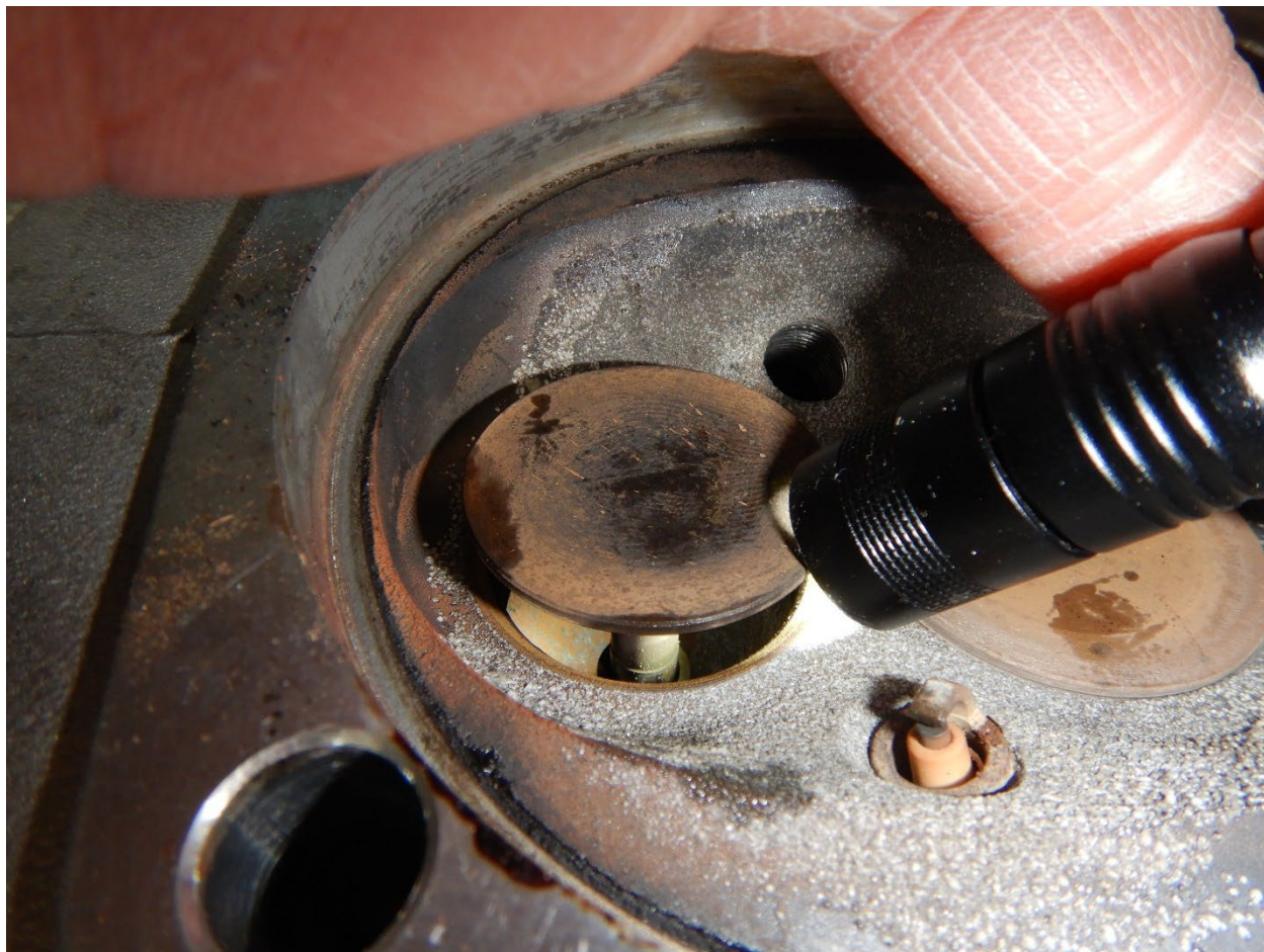
Figure 7. Number 1-cylinder exhaust valve.
