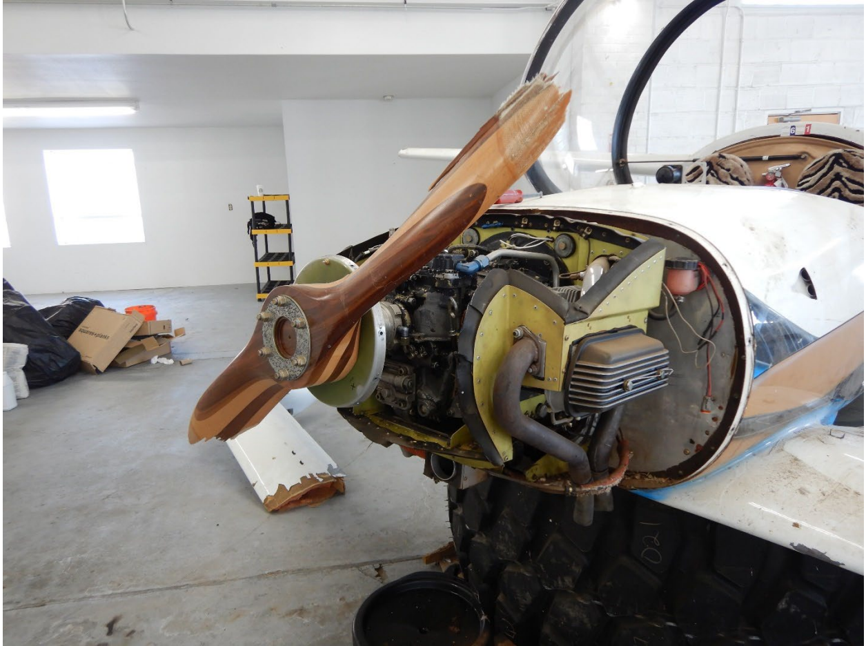
Figure 3. Left-side view of engine showing valve cover for the number 1- and 2-cylinders valve cover.
