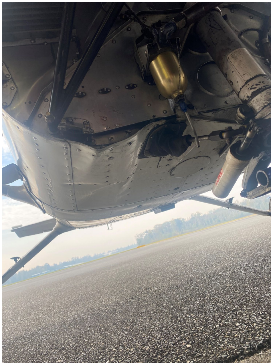
Photo 2 – View of Firewall Damage (Courtesy of Flight School)
