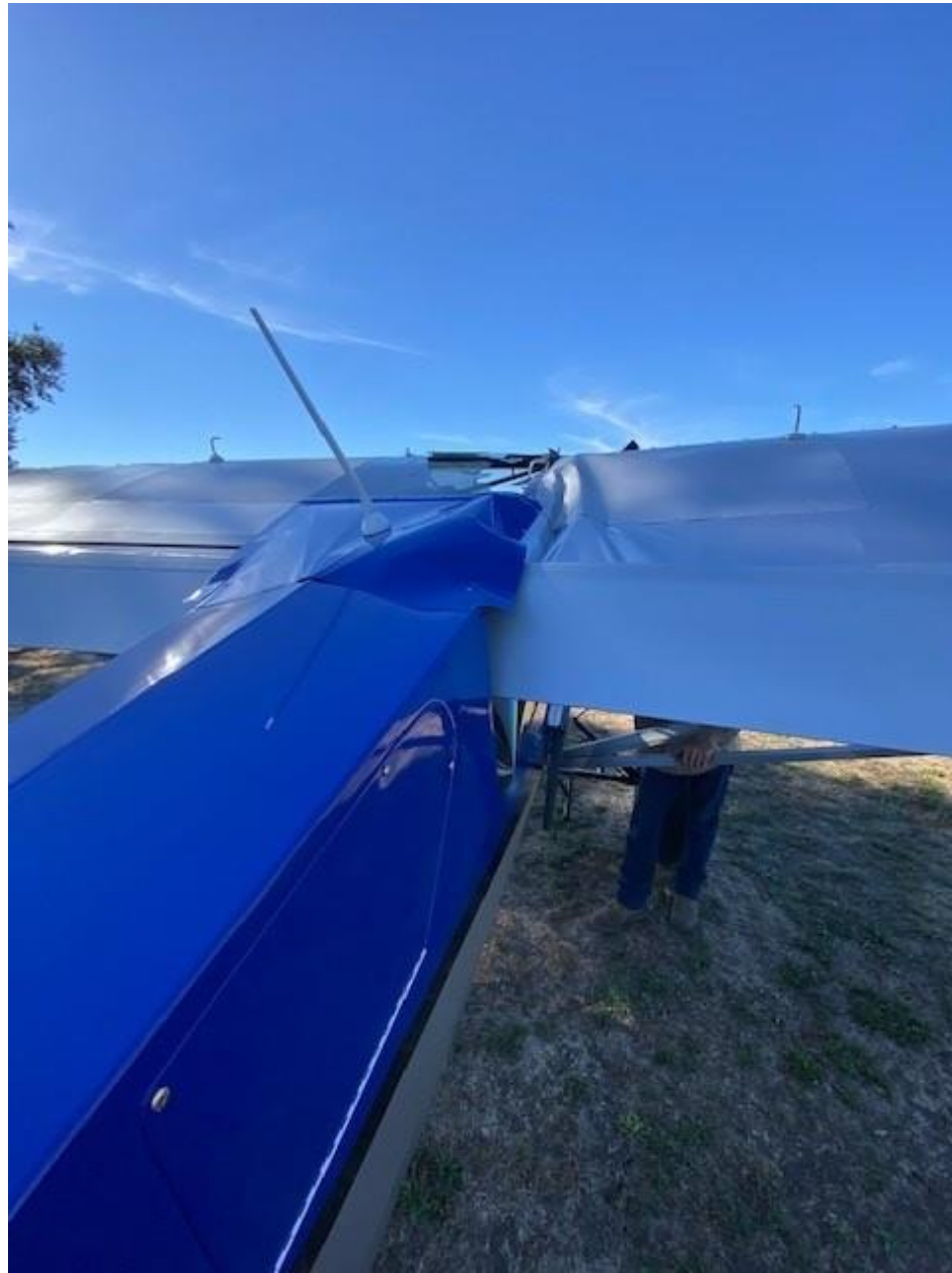
Photo 2 – Accident site, damage to the right wing and fuselage. (Courtesy of the pilot)
