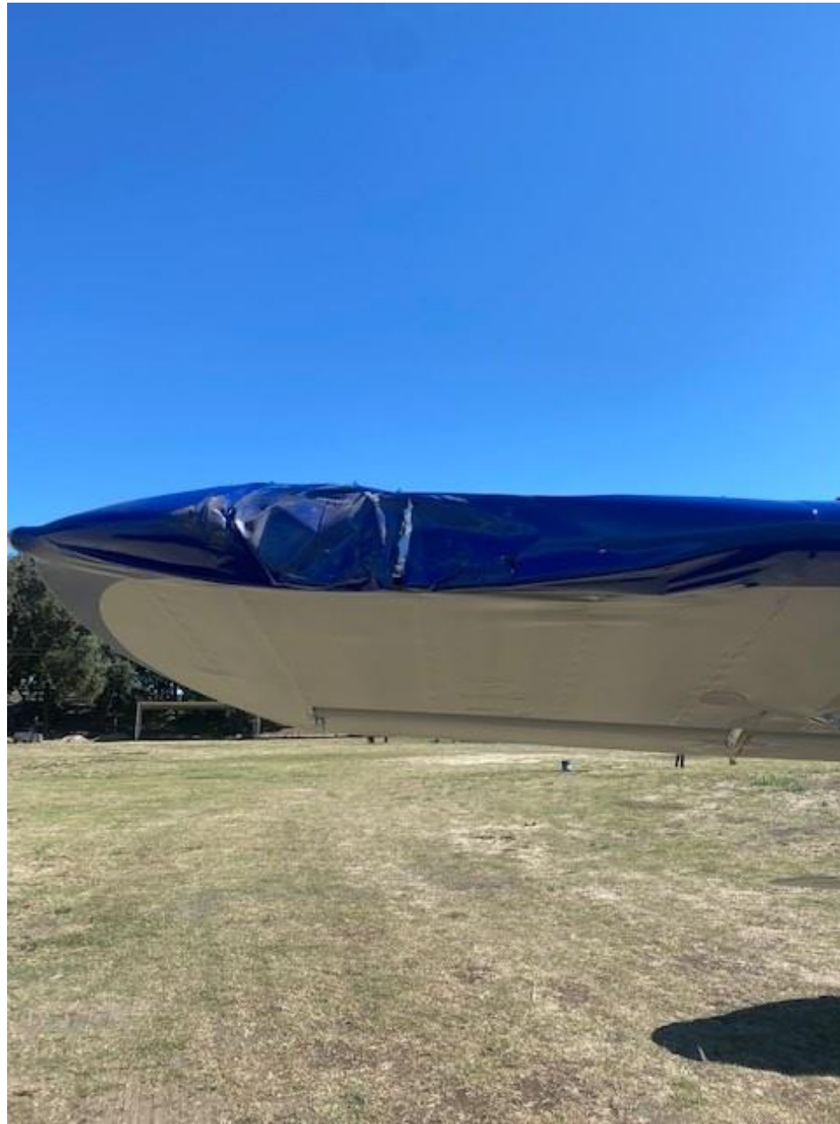
Photo 1 – Accident site, damage to the right wing. (Courtesy of the pilot)
