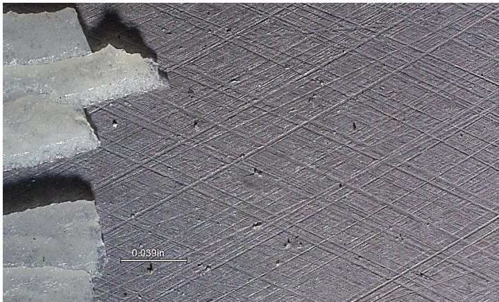
Fixed adapter inner surface showing criss-cross 1 surface finish scratch pattern, similar to an "X" pattern.
