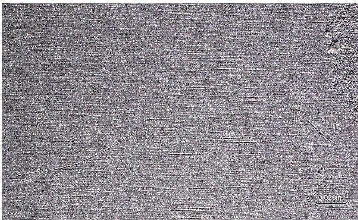
Drive shaft inner surface at the fixed adapter end showing uniform circumferential surface finish scratch pattern.
