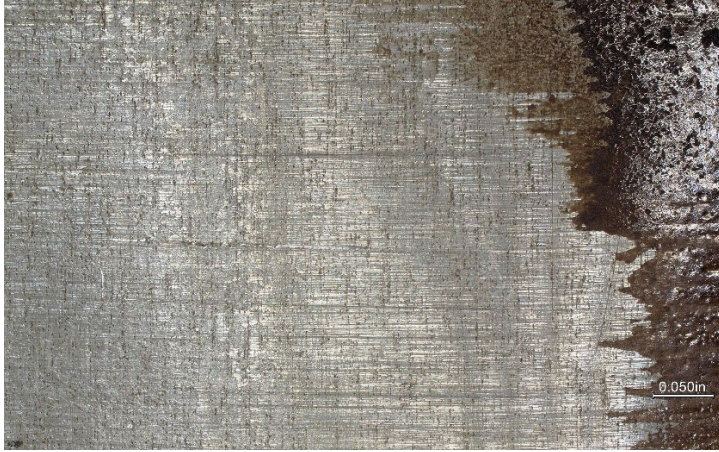
Splined adapter inner surface showing uniform circumferential surface finish scratch pattern.
