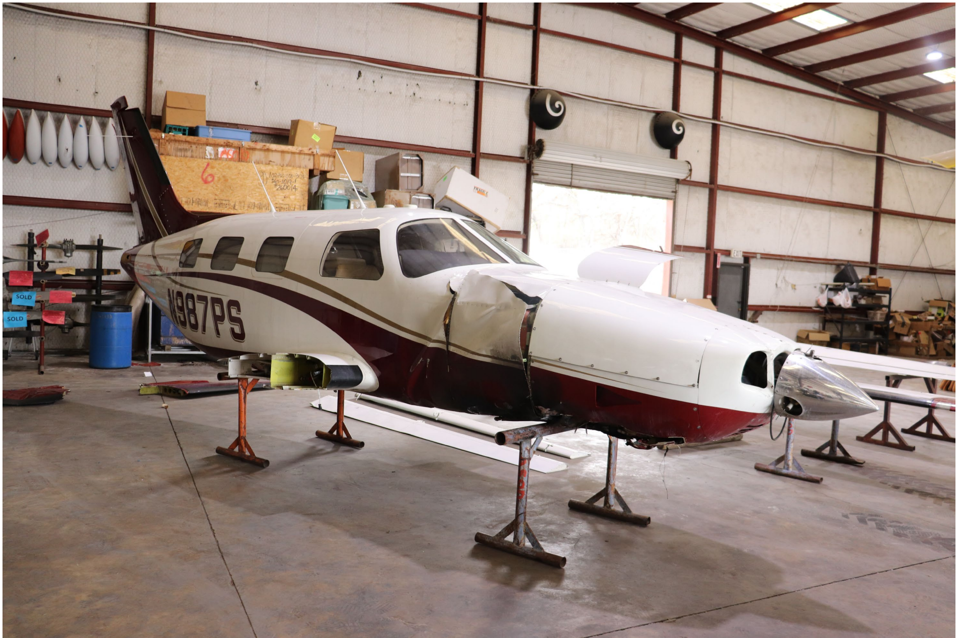
Photo 2 – View of forward fuselage damage
