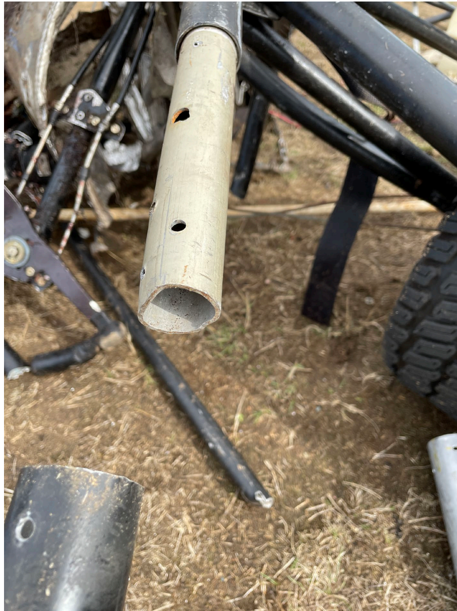
Photo 5 – Spliced wing strut attachment and sleeve
