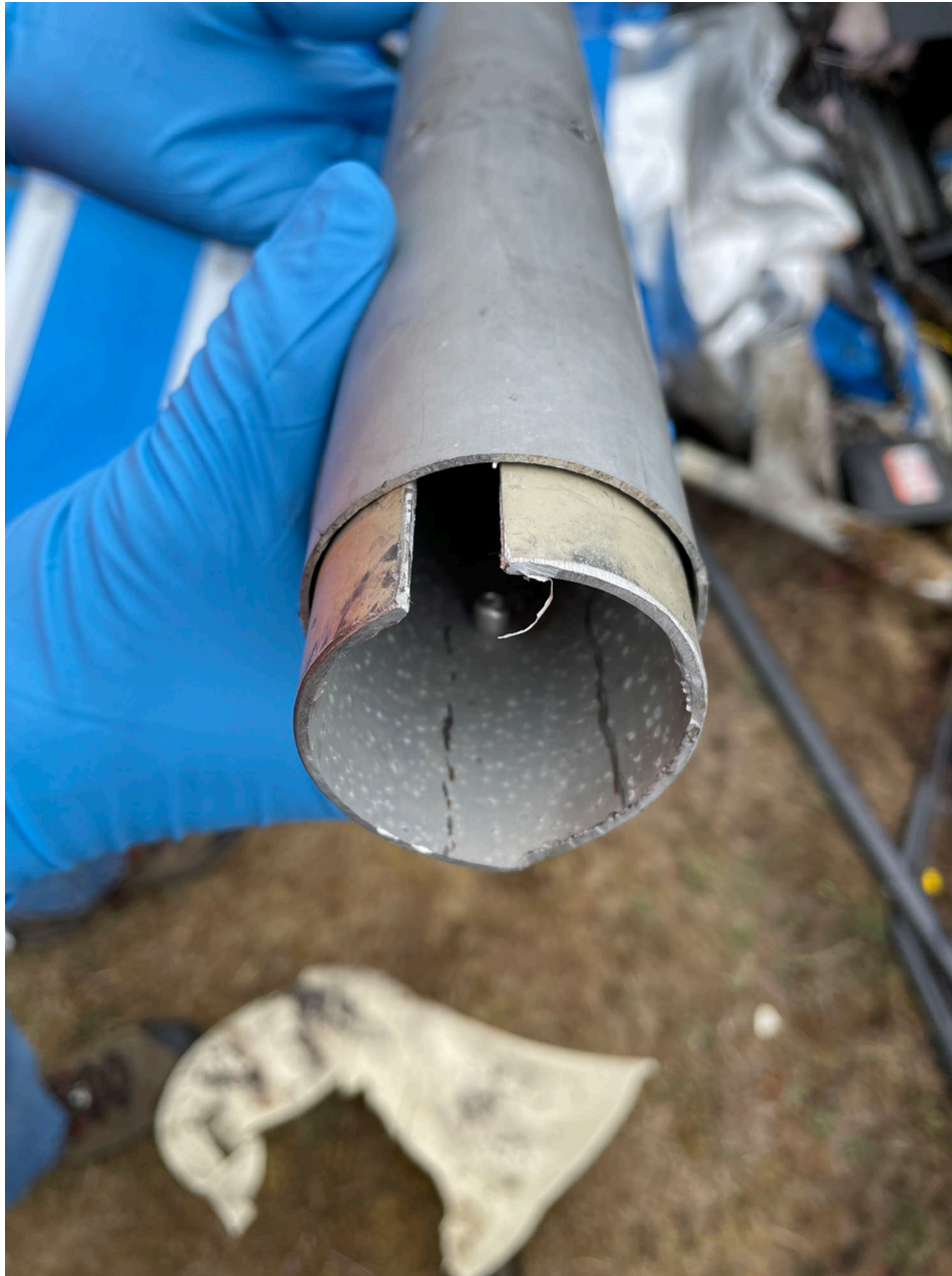
Photo 4 – Spliced wing spar and sleeve
