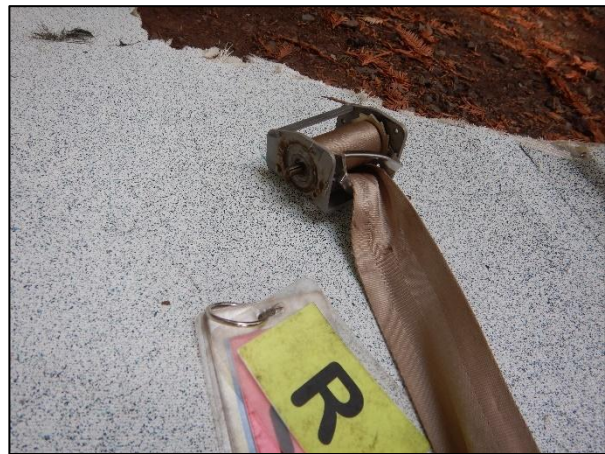
Figure 6. Right forward seat shoulder harness inertia reel.
