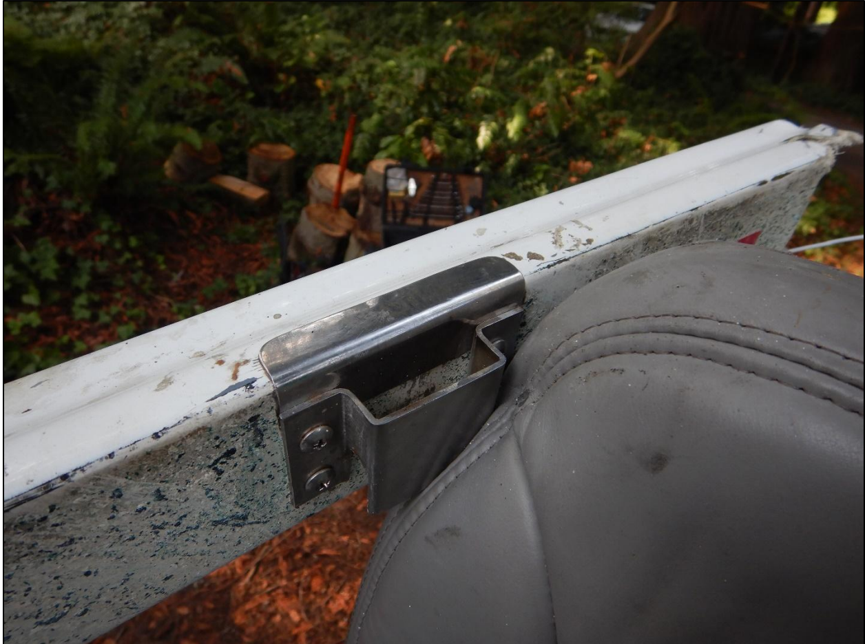
Figure 7. Left canopy latch receiver location.
