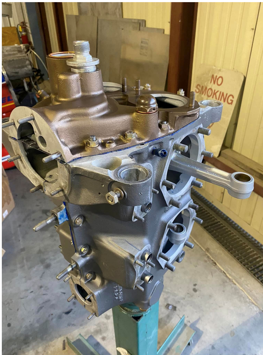
Photo 3 – Engine, accessory case, and connecting rods after coating on July 8, 2023 (pilot's social media page)
