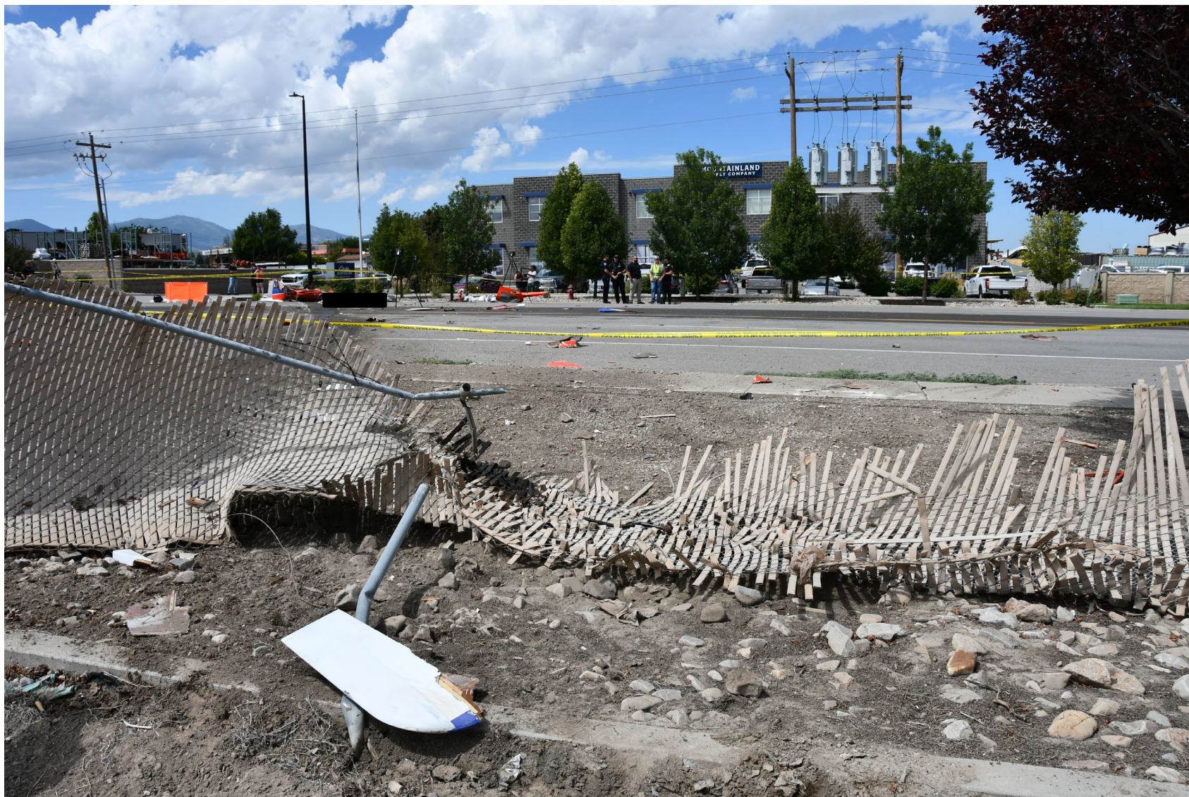
Photo 4 – Separated section of propeller blade at first point of impact with main wreckage in background (courtesy of West Jordan Police Department)
