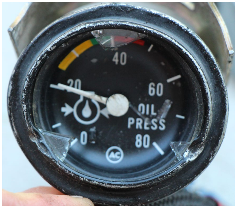
Photograph 8: Oil pressure gauge
