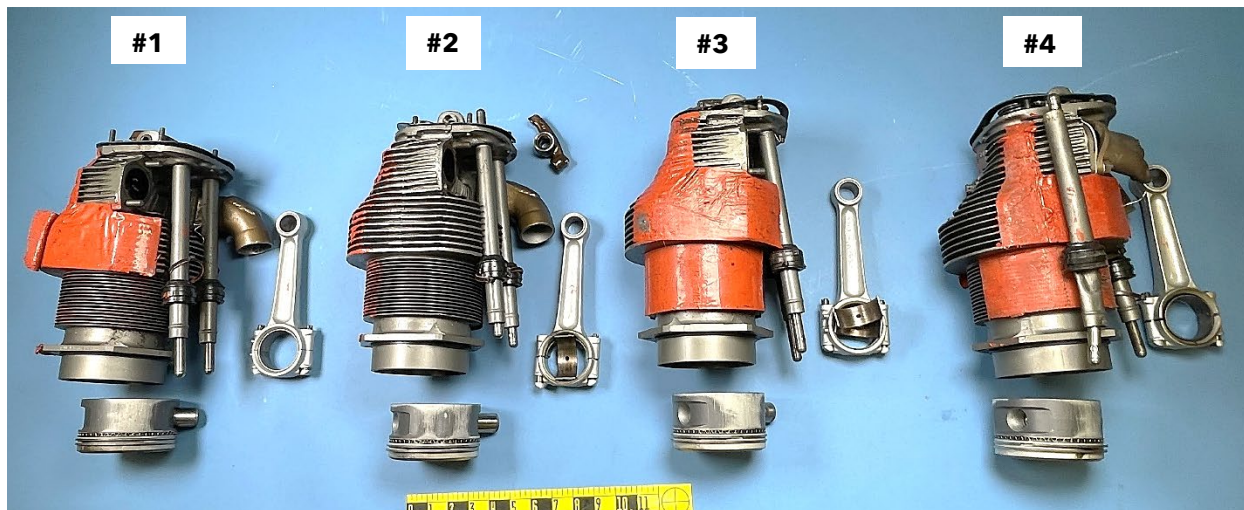
Figure 2. As-received cylinders, connecting rod arms with bearing shells, and pistons with corresponding wrist pins, numbered #1 through #4 (left to right).
