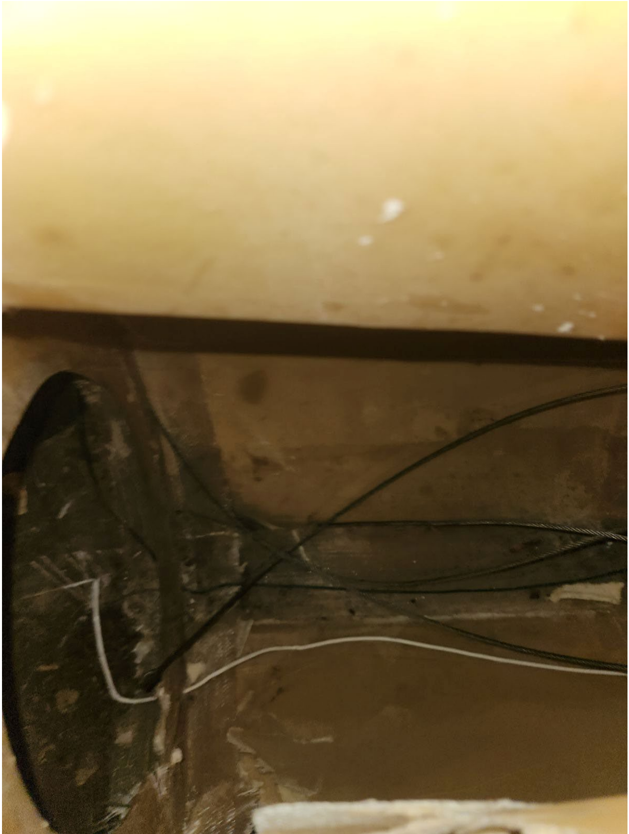
Figure 21. Rudder control cables.
