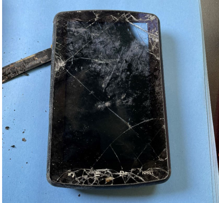
Figure 3. Garmin Aera 796 as received by the vehicle recorder laboratory.
