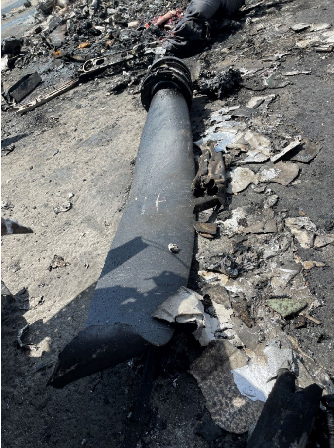
Photograph 10 - Propeller Blade in Main Wreckage
