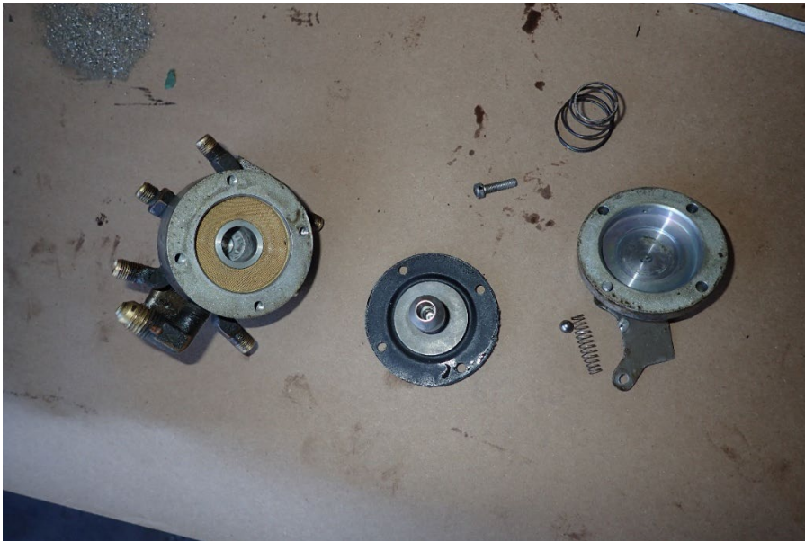
Figure 8. Fuel Metering Assembly (Photo Courtesy of Textron Aviation)
