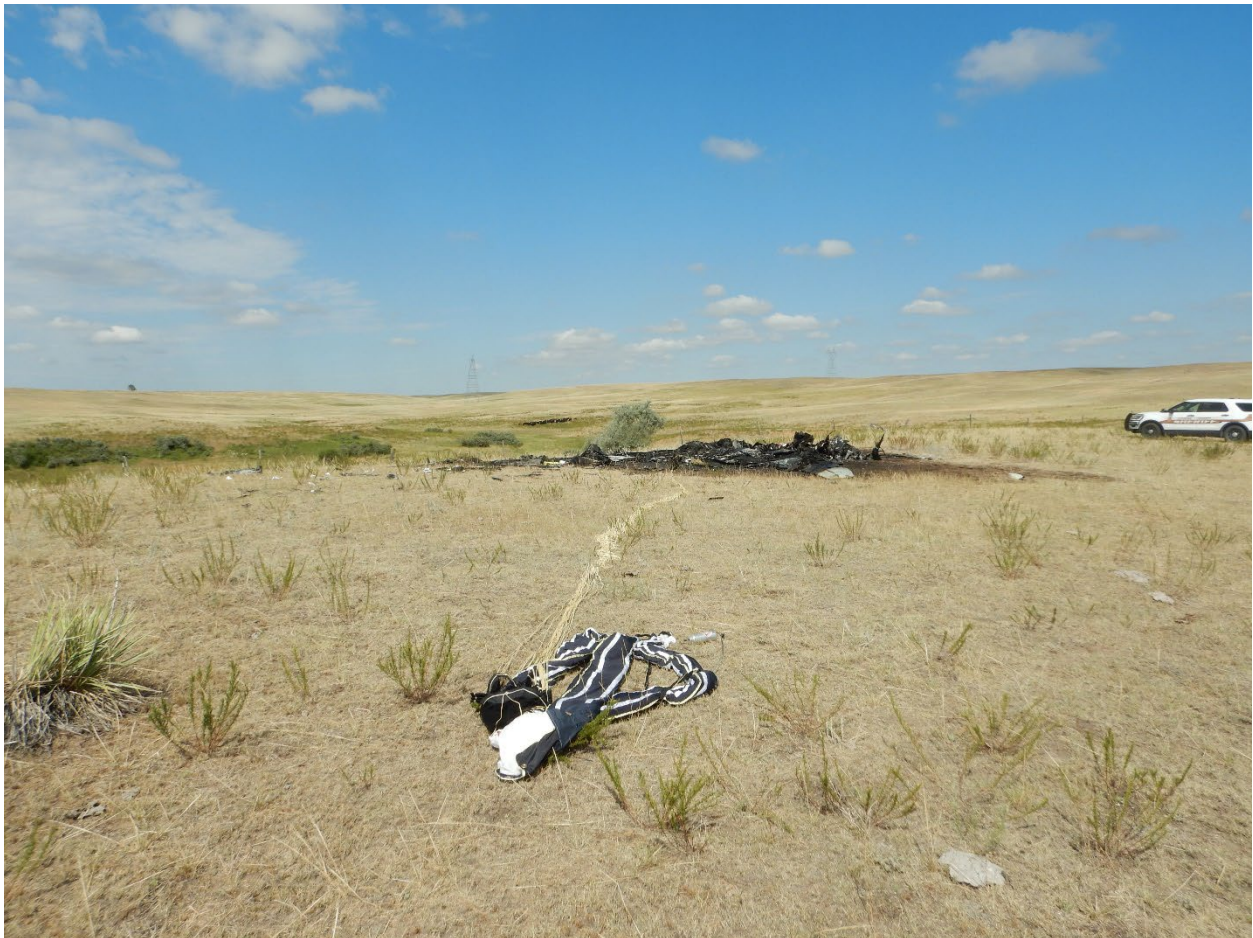
Photograph 2: North view with deployed airframe ballistic parachute
