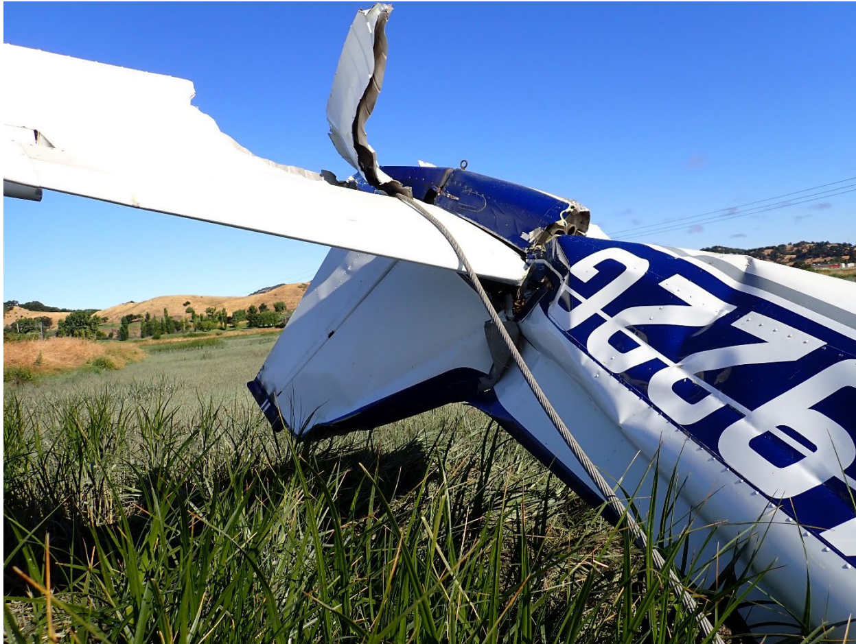
Photograph 3 - Empennage Wrapped with Power Line (Courtesy of Textron Aviation)
