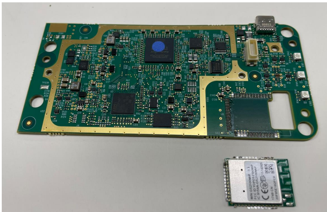
Figure 4. The WiFi module was dislodged from its circuit board as a result of the crash.
