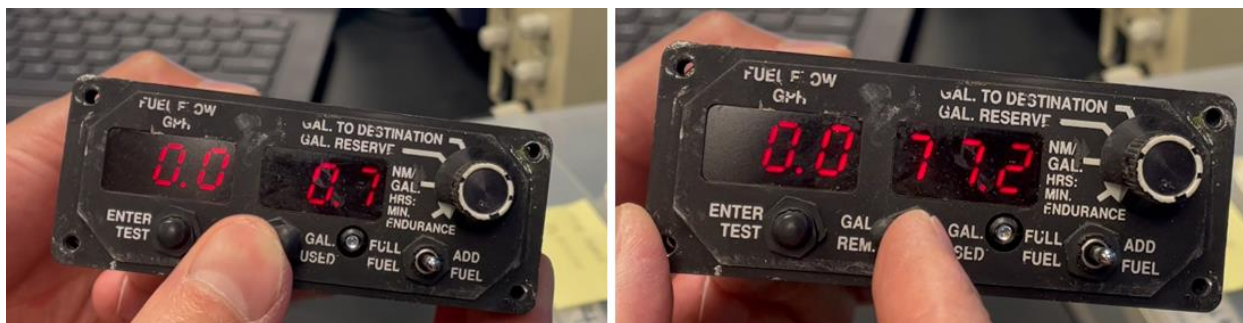
Figure 2. Recorded fuel used data on the left, and fuel remaining data on the right.
