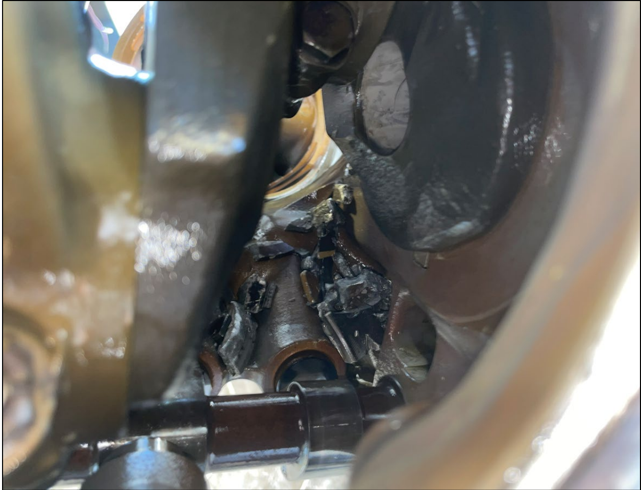
Photo 10. View of metal from cylinder No. 6 piston skirt.
