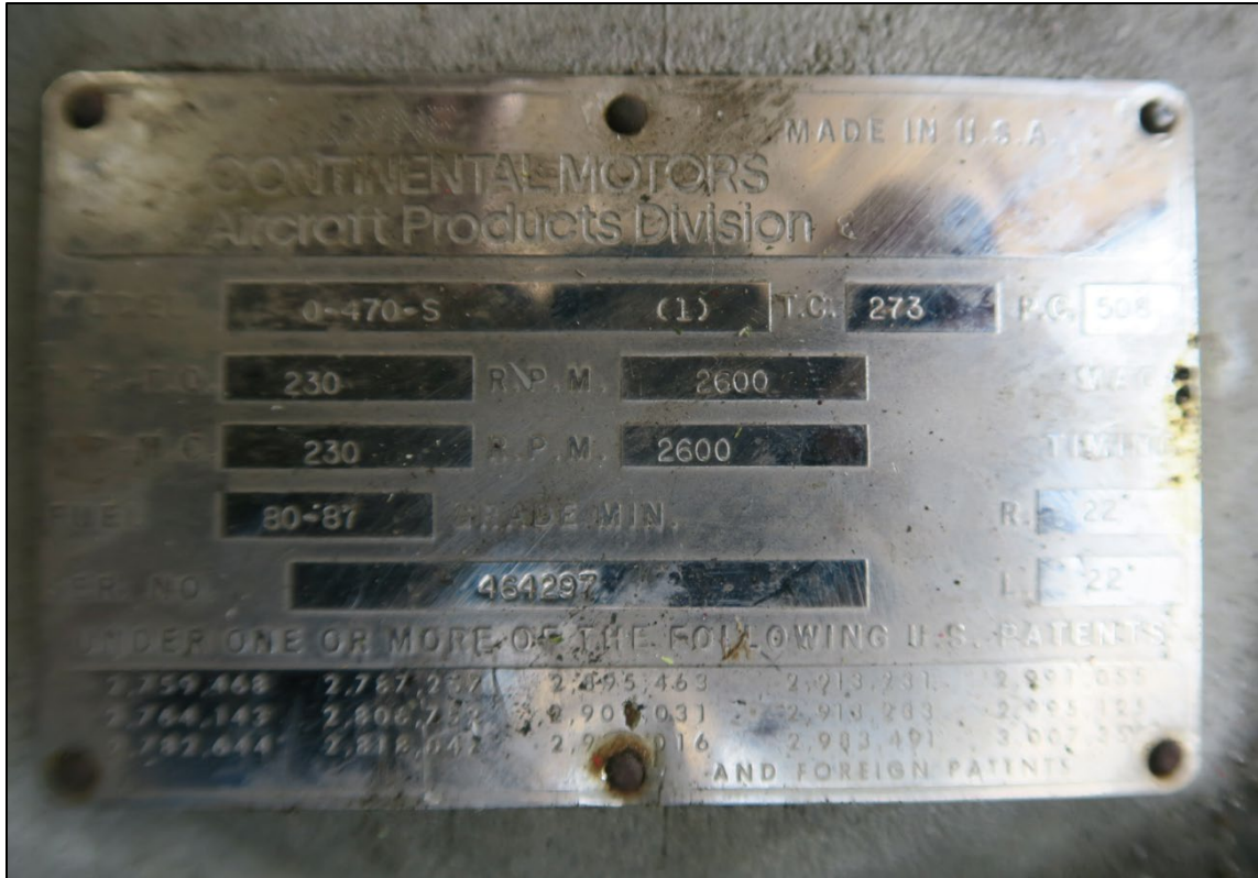
Photo 1. Engine data plate.
