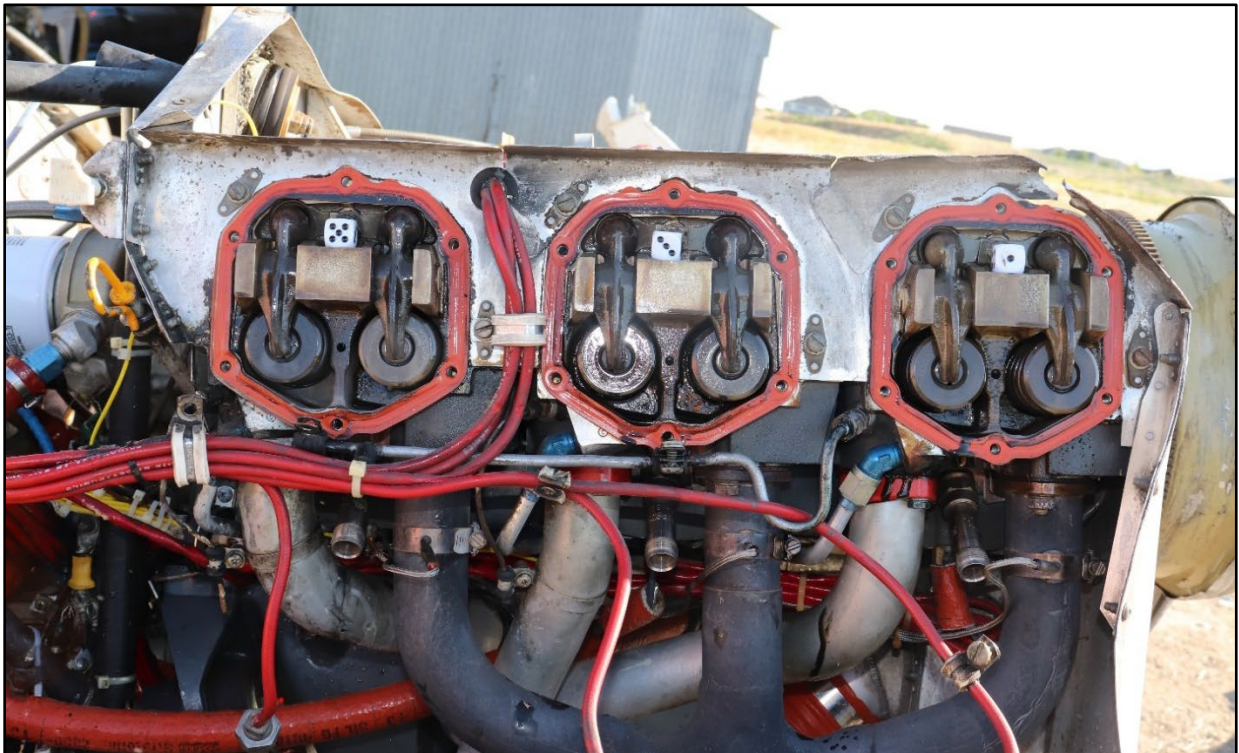
Figure 8: view of right side intake and exhaust rocker arms
