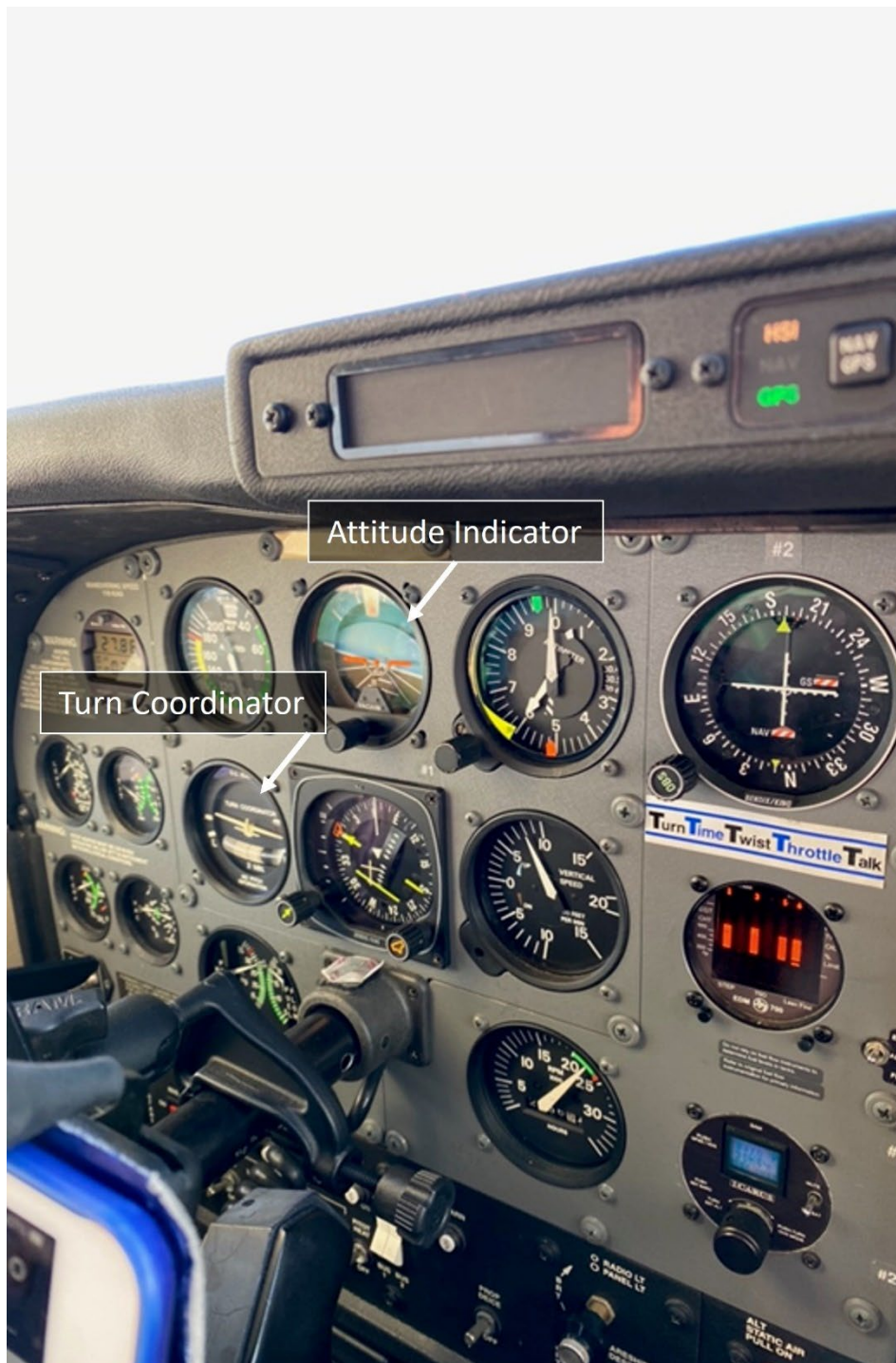
Figure 1. Photo of the accident airplane instrument panel, showing the attitude indicator indicating a left bank while the turn coordinator indicating a right bank. Photo courtesy of the CFII.
