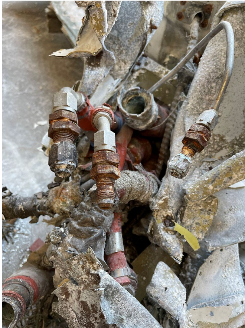
Photograph 8 - Fuselage Fittings and B-Nuts (Courtesy of NTSB)
