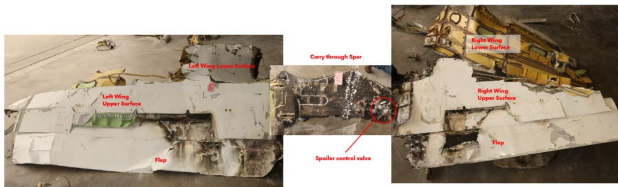
Figure 10. Composite image of both wing sections joined by the wing spar carry through.
