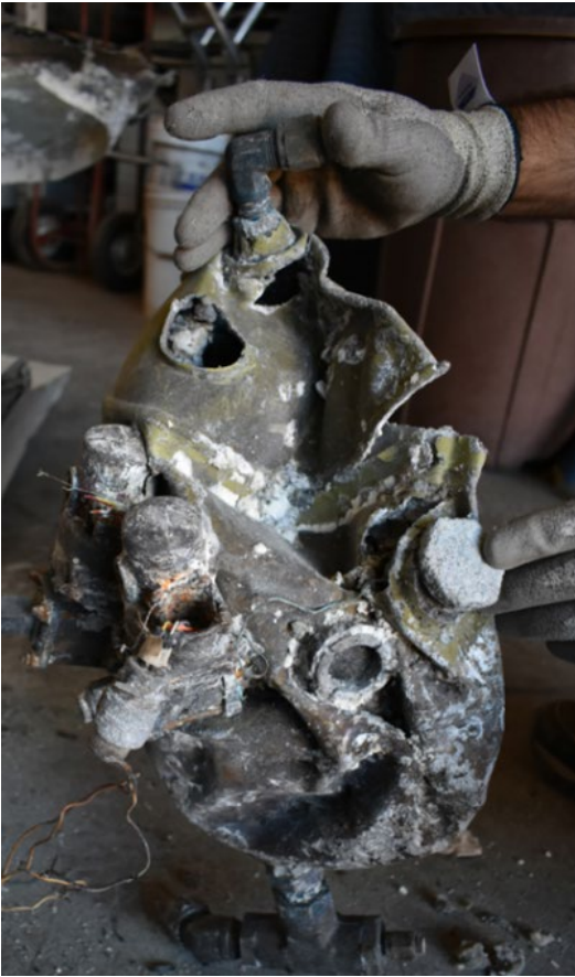
Figure 19. Hydraulic reservoir, inward facing quadrant.
