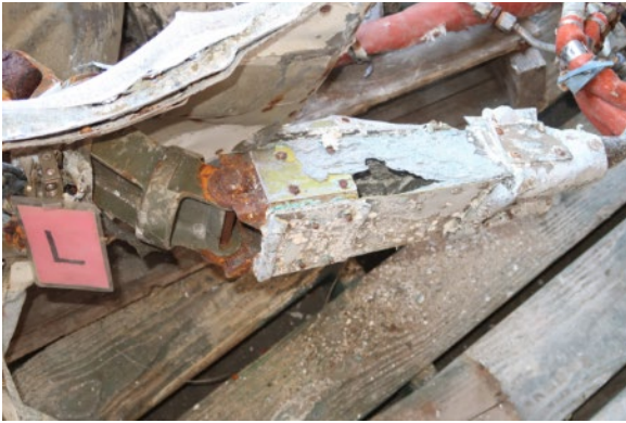
Figure 14. Left rear engine mount beam.
