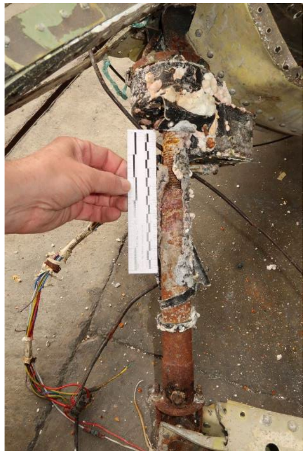
Figure 8. Elevator trim jack screw.
