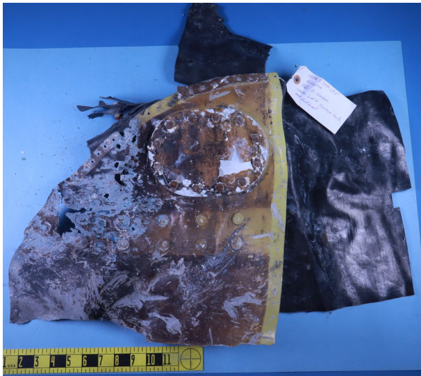
Figure 4. Left side top portion of the fuselage fuel tank aft bulkhead.
