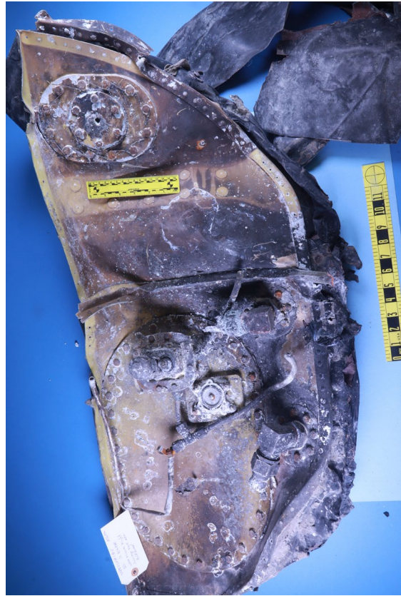
Figure 3. Right side portion of the fuselage fuel tank aft bulkhead.
