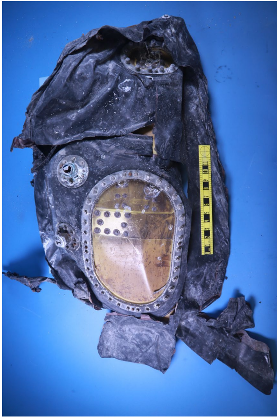
Figure 3. Right side portion of the fuselage fuel tank aft bulkhead.
