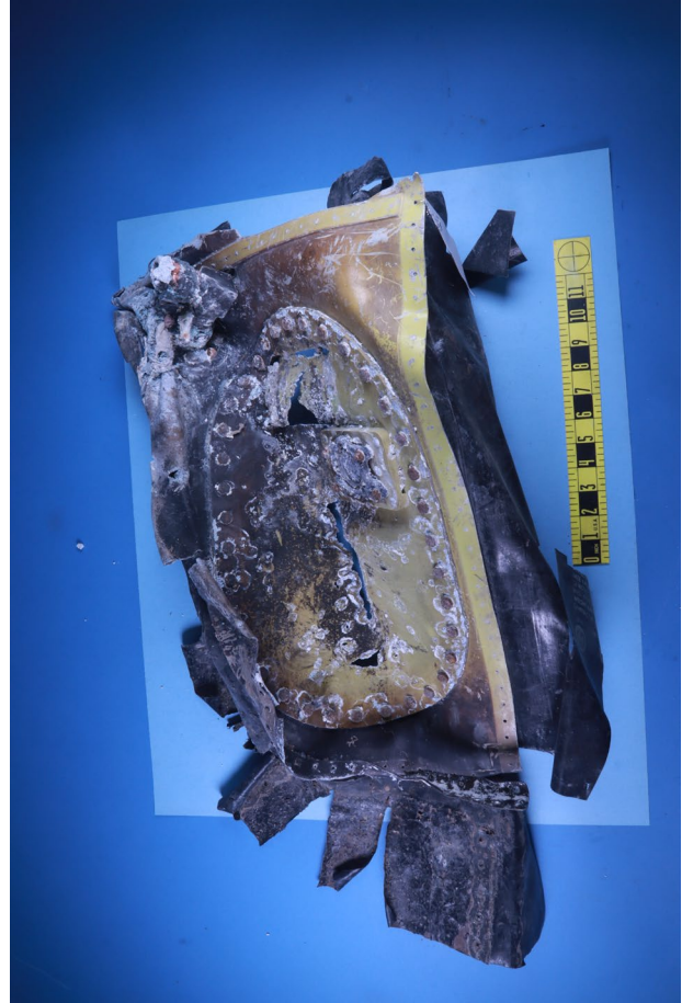
Figure 5. Left side bottom portion of the fuselage fuel tank aft bulkhead.
