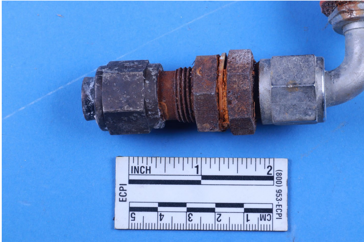
Figure 13. Hydraulic fluid return line bulkhead fitting.
