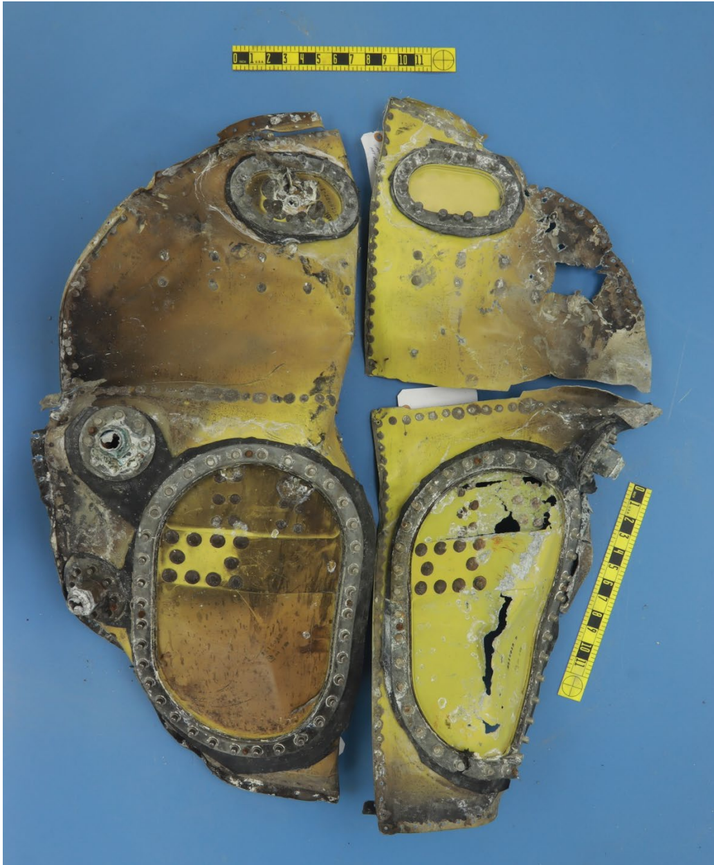
Figure 11. Forward-facing side of the fuselage fuel tank aft bulkhead with the rubber fuel tank liner removed.
