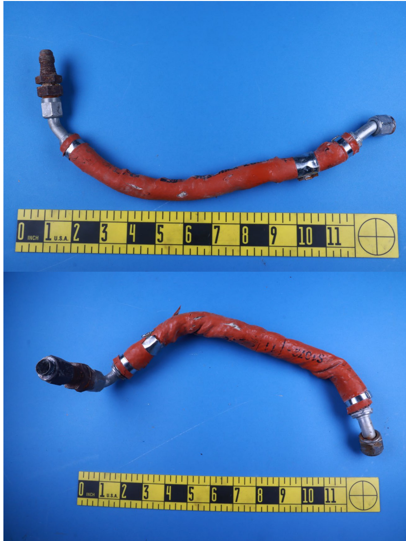
Figure 2. Motive flow fuel line with fittings (Top) Hydraulic fluid return line with fittings (Bottom) as received.
