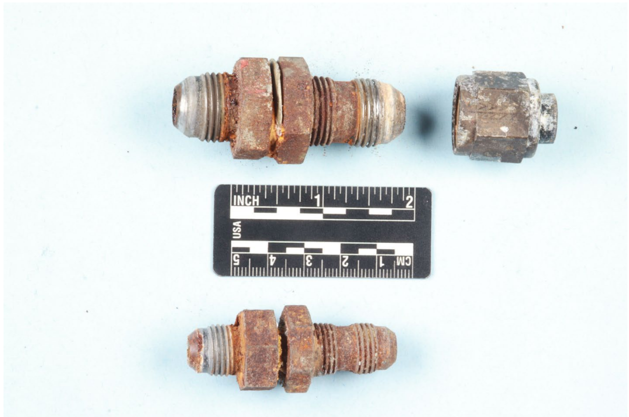
Figure 14. Hydraulic fluid return (top) and motion flow fuel fitting (Bottom).
