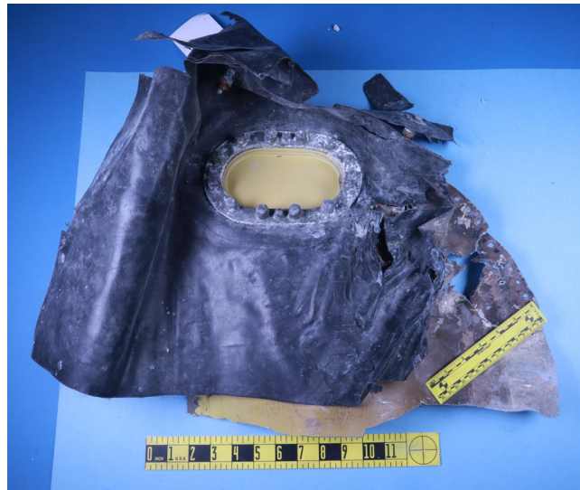
Figure 4. Left side top portion of the fuselage fuel tank aft bulkhead.
