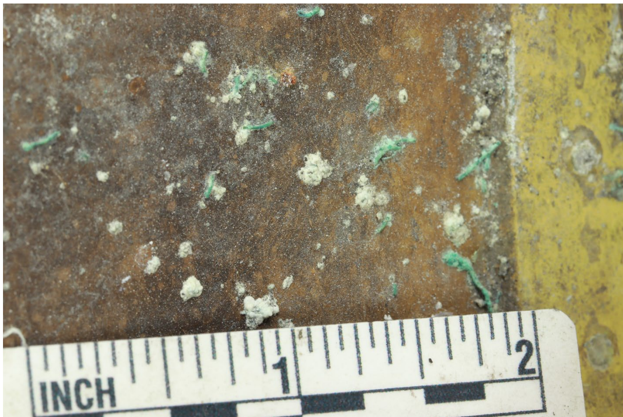
Figure 9. Green debris adhering to the aft-facing surface of the right-side portion of the fuselage fuel tank aft bulkhead.
