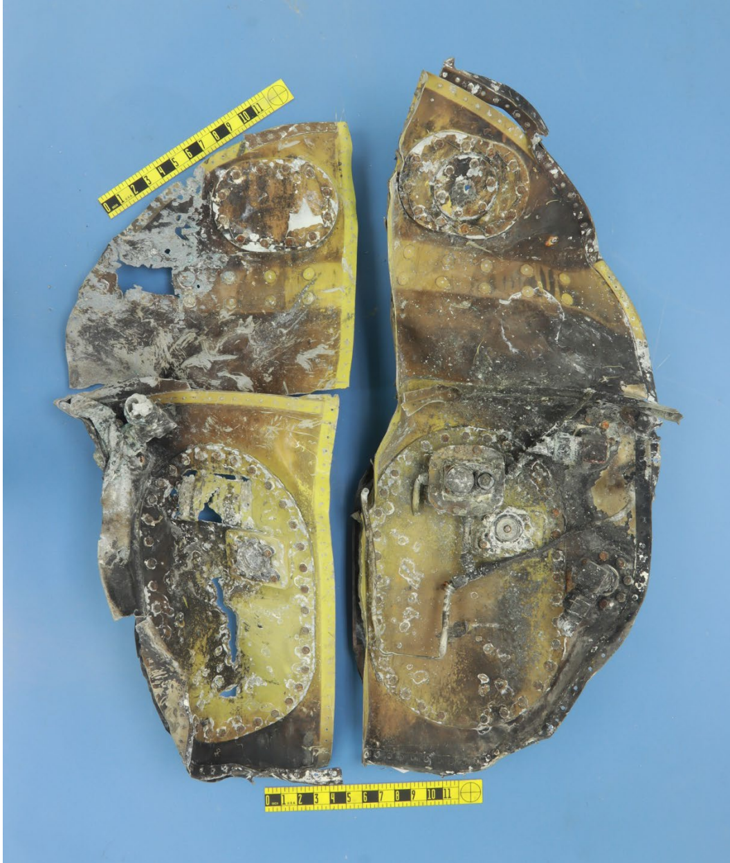
Figure 10. Aft-facing side of the fuselage fuel tank aft bulkhead.
