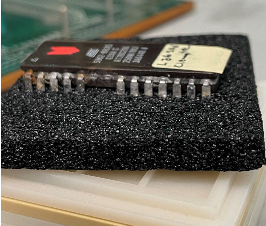
Photo 6, Missing Contact Pins
