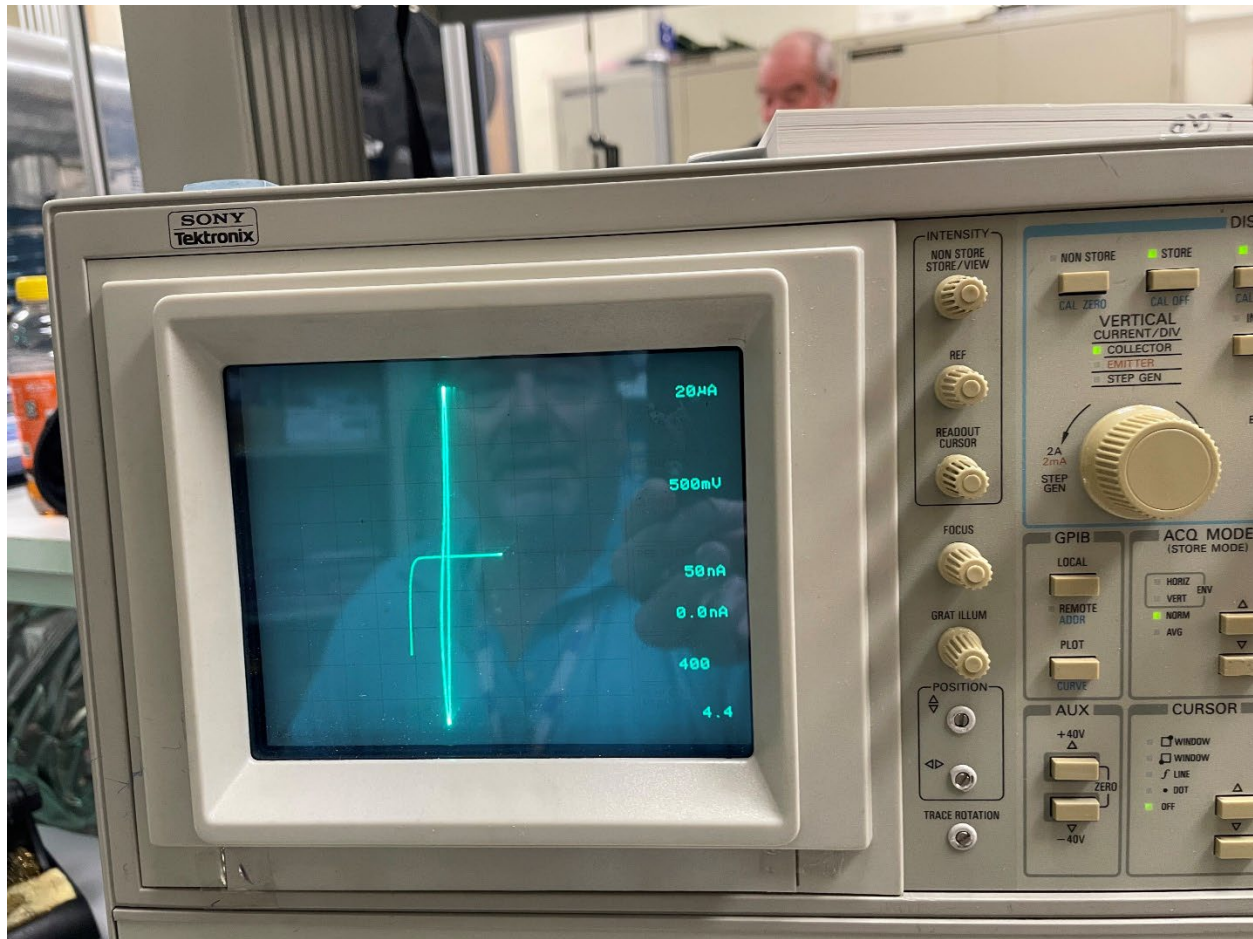
Photo 8, Curve Tracer Display showing one channel (narrow vertical loop) on the Accident Chip (The proper continuity curve display is superimposed)
