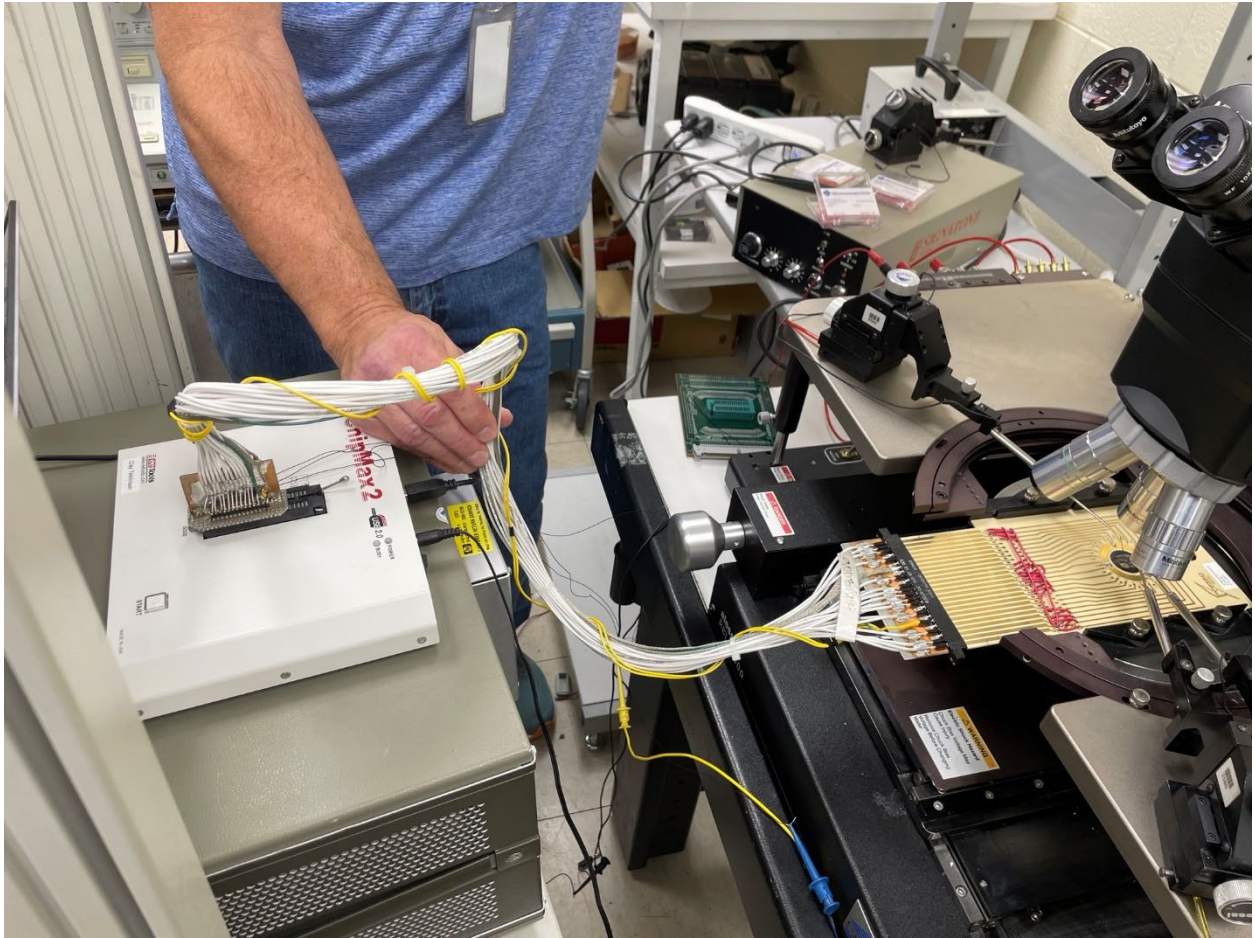
Photo 13, Chip Card with Microprocessor, Wire Harness from Chip Card to Canon Plug, Plugged into the Chip Reader.
