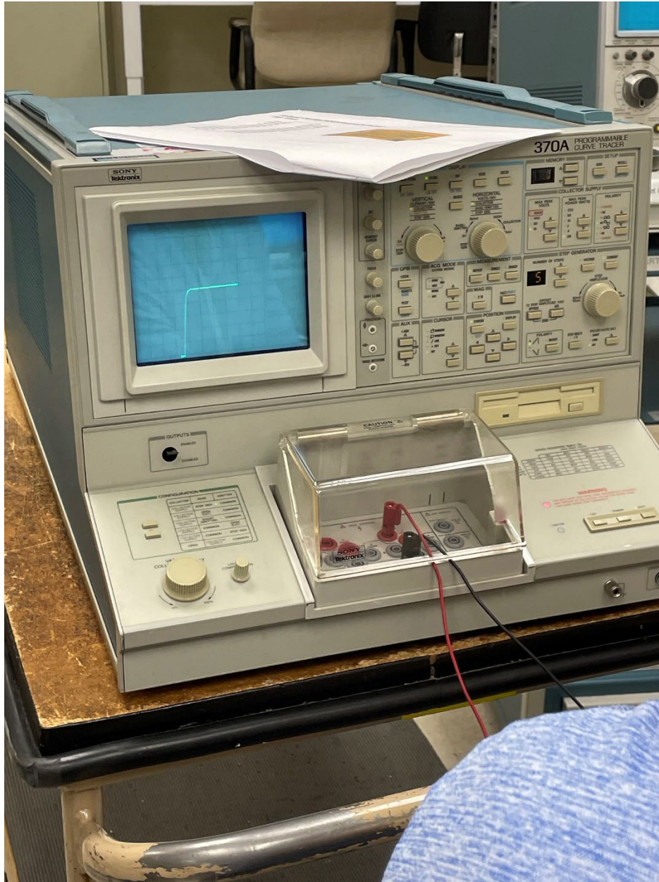
Photo 12, Second Curve Trace showing Microprocessor Continuity
