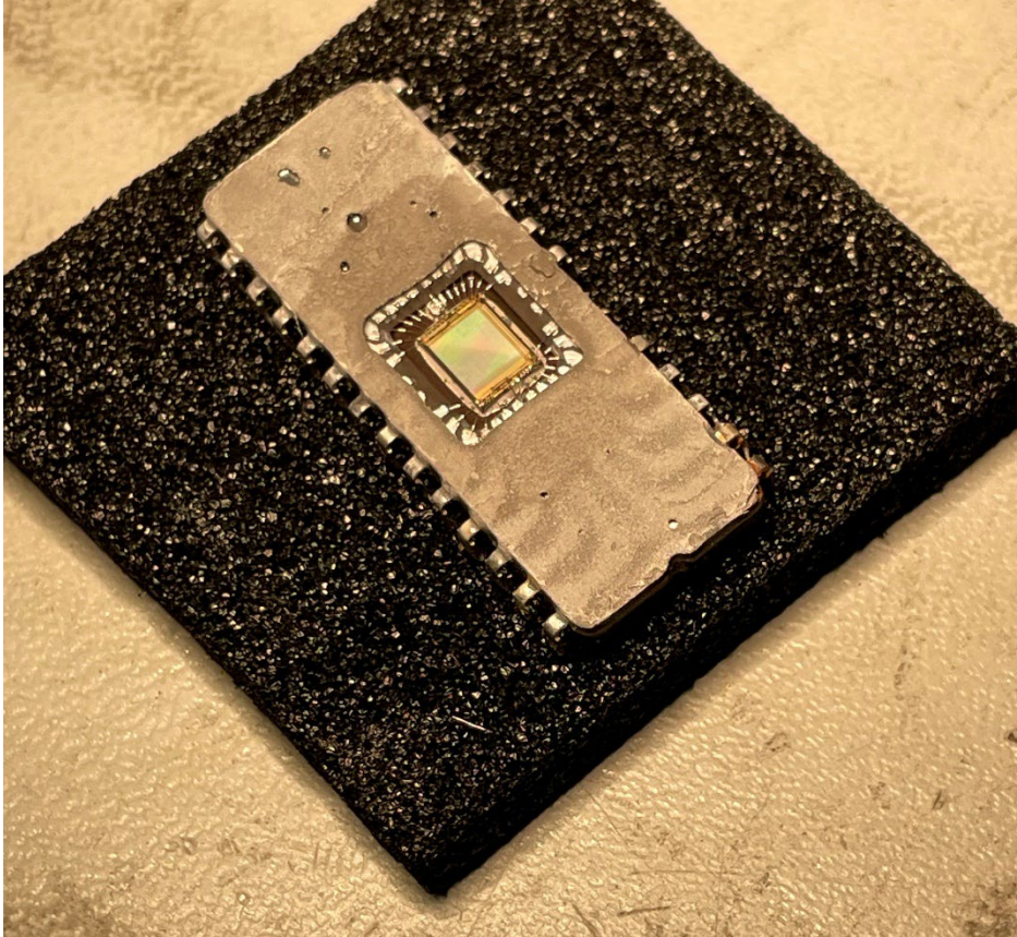
Photo 9, Opened Accident Microchip Showing the Microprocessor in the Center
