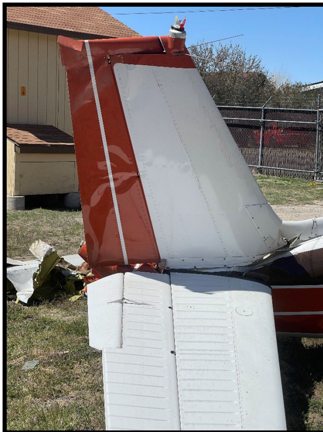
Figure 4: View of damage to horizontal stabilizer and rudder
