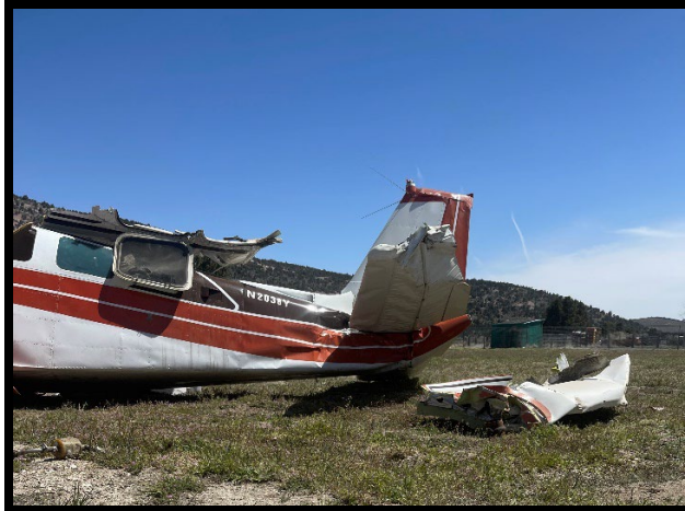
Figure 3: View of empennage damage
