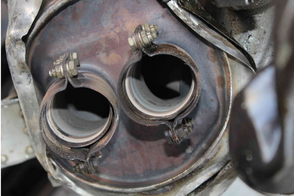
Figure 13 - Exhaust pipe outlets
